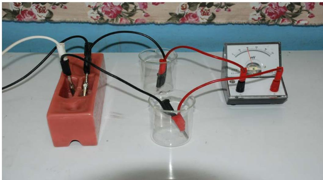
**Figure 2.** Illustration of apparatus for measuring electric current and the dental surface potentials
