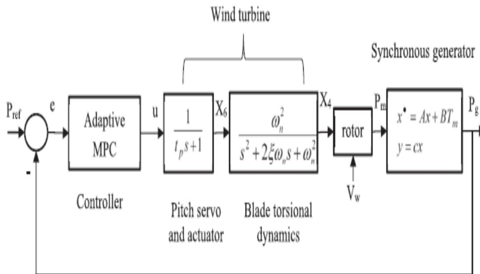
Figure 6. Block diagram of the WT with BPC [10]
