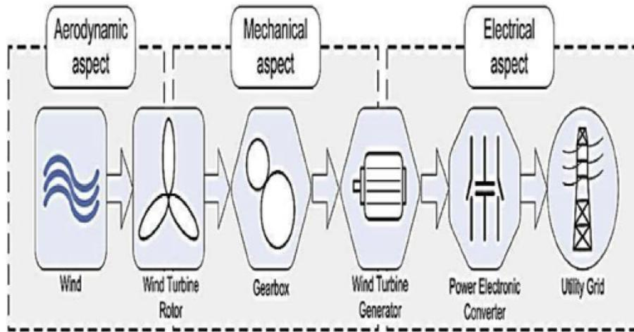
Figure 5. Main elements of wind energy conversion system [10]
