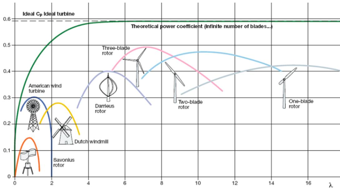
Figure 3. Cp to TSR in different types of wind turbines [5]
