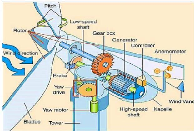
Figure 2. Inside wind turbines [6]
