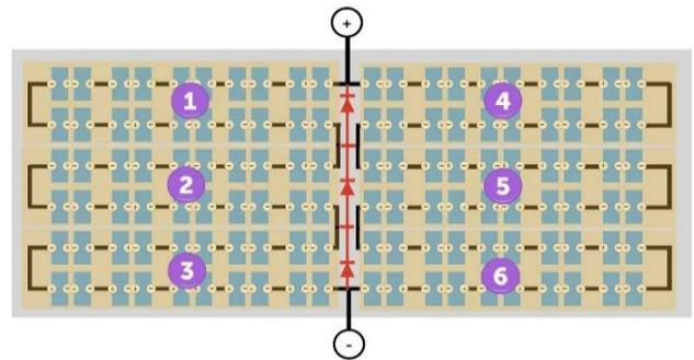
**Figure 9.** Showing how to connect half of the cells [12]
