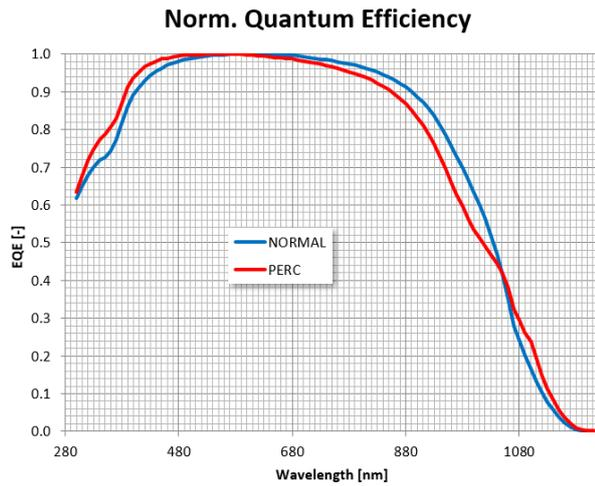
**Figure 7.** Spectral response between a normal solar cell and a solar cell of type PERC [11]
