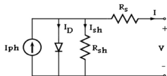
Figure 1. Equivalent circuit of PV cell [4]
