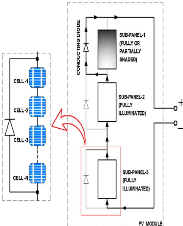
Figure 3. Power flow in PV module under PSC [8]
