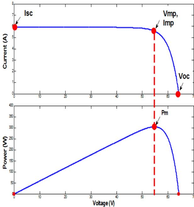
Figure 2. PV module curves under STC (25°C and 1000W/m<sup>2</sup>) [4]
