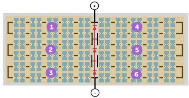
**Figure 8.** Showing how the normal cells in the solar panels are serially connected and form three lines [12]
