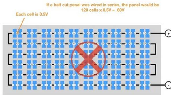
**Figure 11.** The correct half-cell conduction and how voltage is distributed across cells [12]
