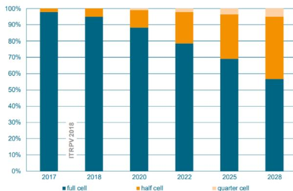
**Figure 12.** Different cell dimensions in c-Si modules [12]
