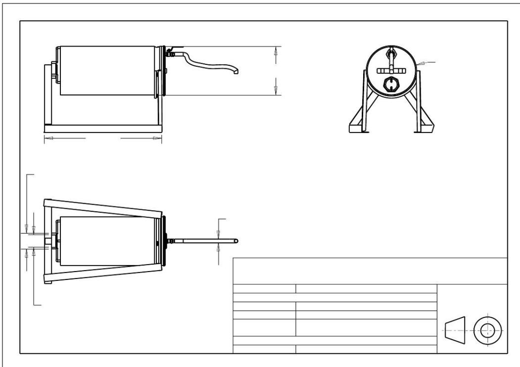
Figure 1. Orthographic views of the designed biogas digester on its mountings
