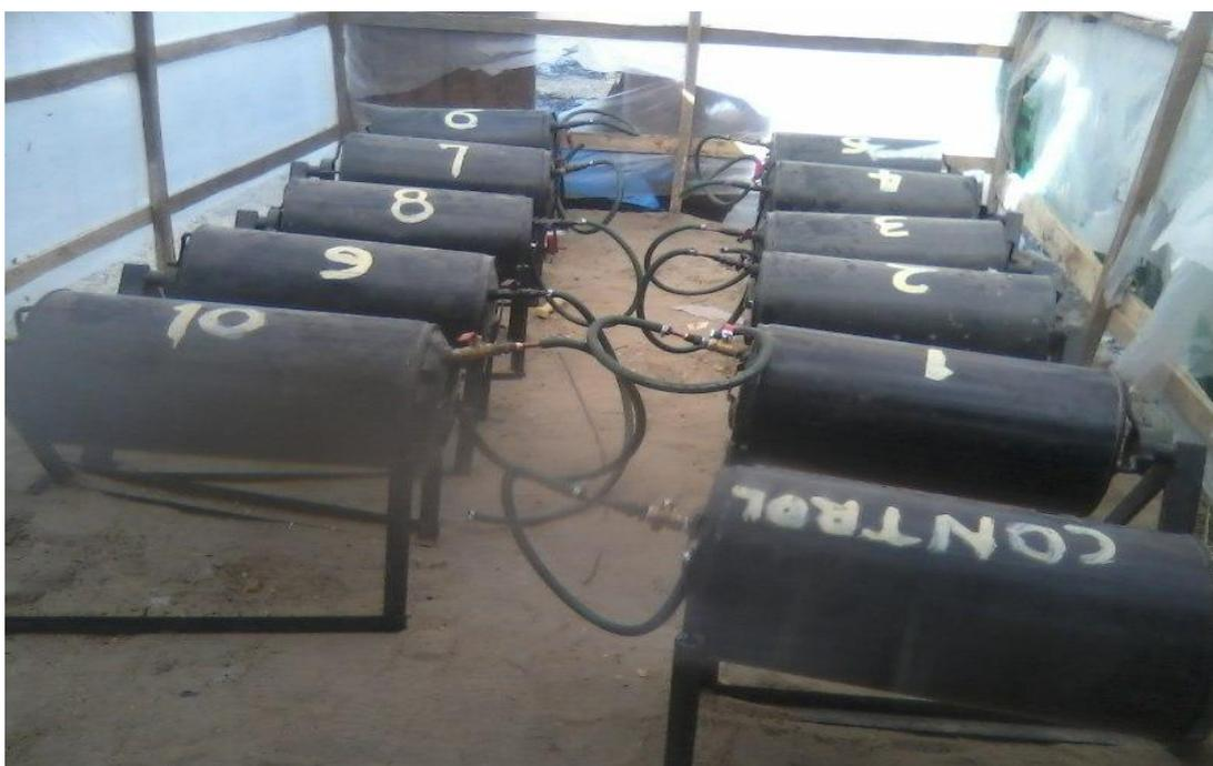
**Plate 1.** Arrangement of the biogas digesters in the greenhouse-like structure
