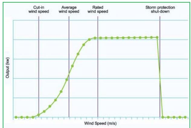
Figure 3. Idealized wind turbine power curve [7]
