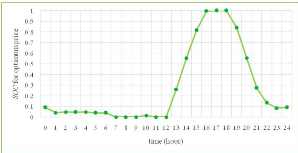
Figure 11. Simulation results for hourly variations of battery state of charge (SOC) in case I
