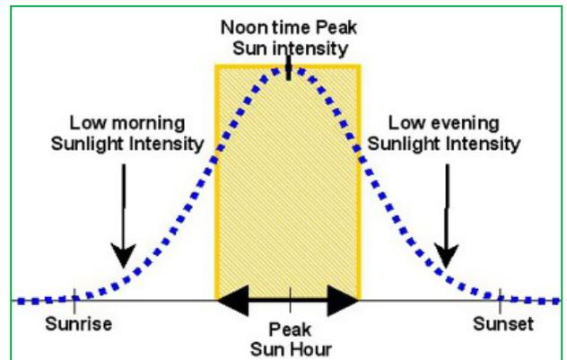
Figure 2. Typical electricity PV generation profile [6]
