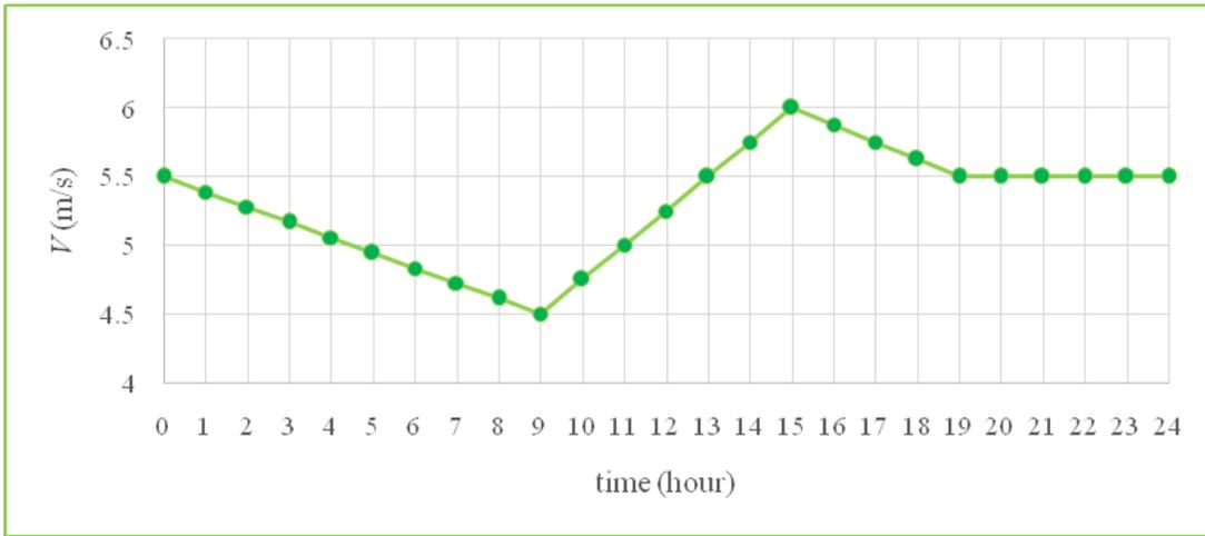
Figure 5. Distribution of daily wind speed at turbine height used for the turbine power output [11]
