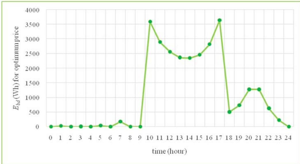
Figure 9. Simulation results for hourly variations of power flow into the balance boundary of the building through battery storage in case I
