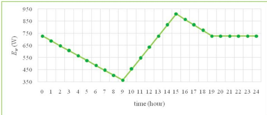
Figure 8. Distribution of daily wind turbine power used in the model
