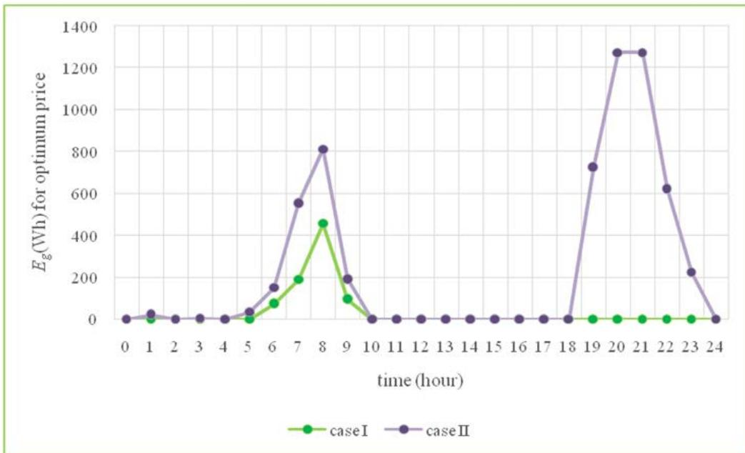
Figure 10. Simulation results for hourly variations of power flow into the balance boundary of the building through electricity grid in cases I and II
