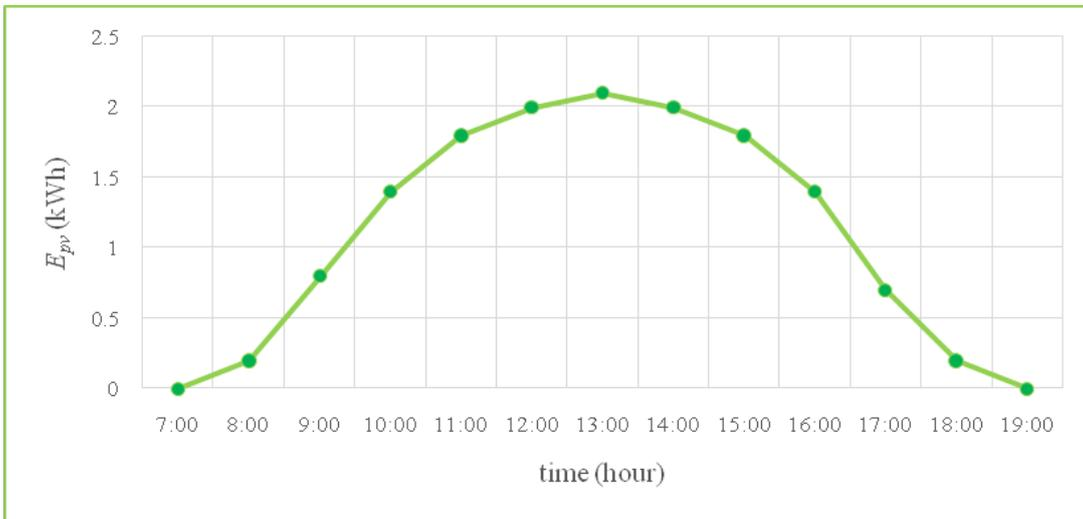
Figure 6. Distribution of hourly photovoltaic energy generation [12]
