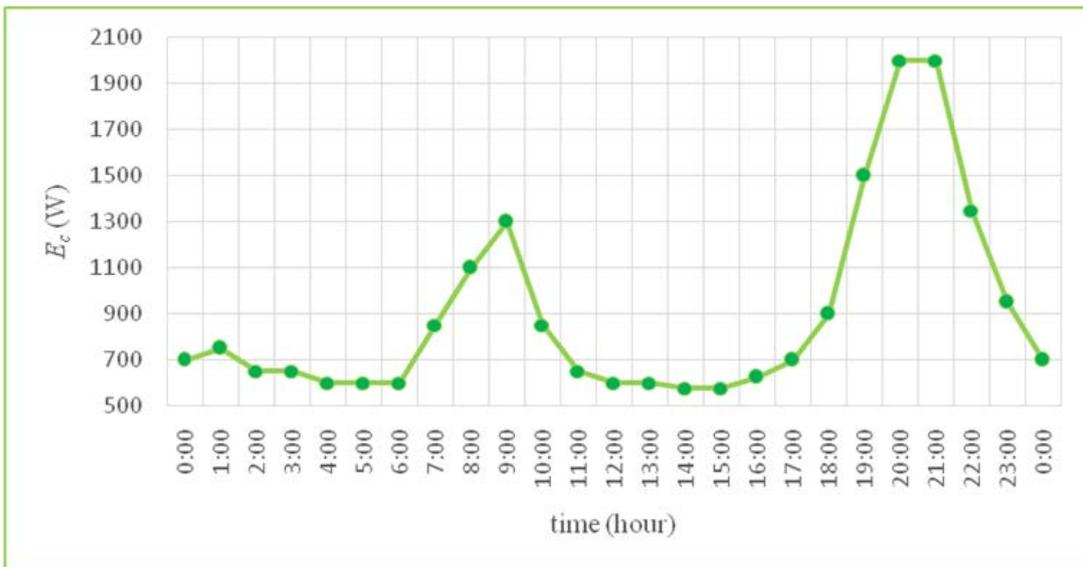
Figure 7. Distribution of hourly energy consumption for a typical family [13]
