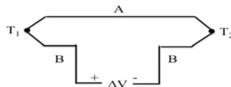
Seebeck effect: A temperature difference create a potential difference for the junction between materials A and B.
