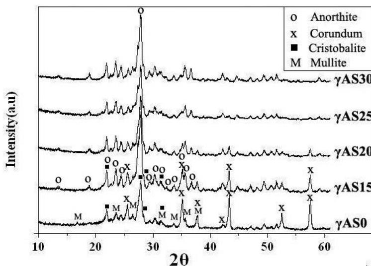
**Figure 3.** XRD patterns of (γAS0) and γ-Alumina bodies containing air blast furnace slag at vitrified temperature**Table 5. Real intensity of crystalline constituents and electrical properties of base composition (γAS0) and/ γ-Alumina bodies containing air blast furnace slag**
