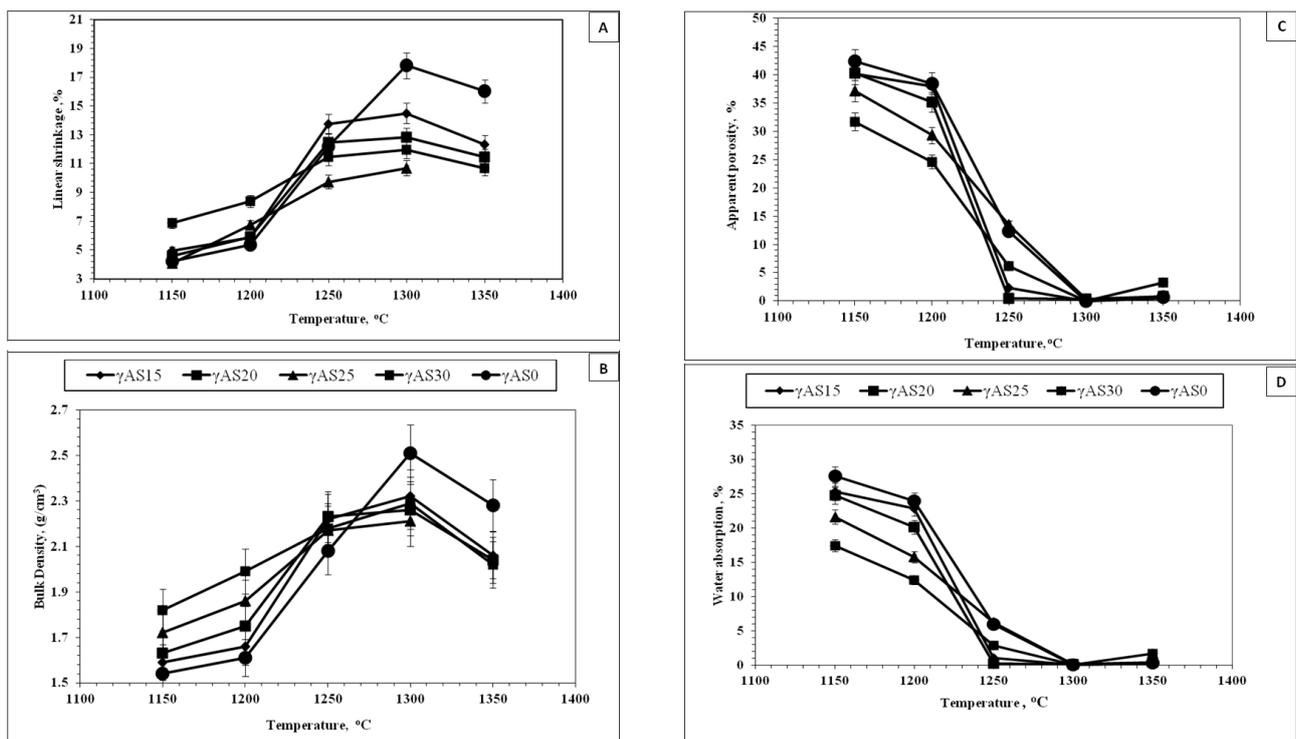
**Figure 2.** Physical properties of base composition ( $\gamma$ AS0) and  $\gamma$ -Alumina bodies containing air blast furnace slag at different sintered temperatures, (A) linear shrinkage, (B) Bulk density, (C) Water absorption, (D) Apparent porosity
