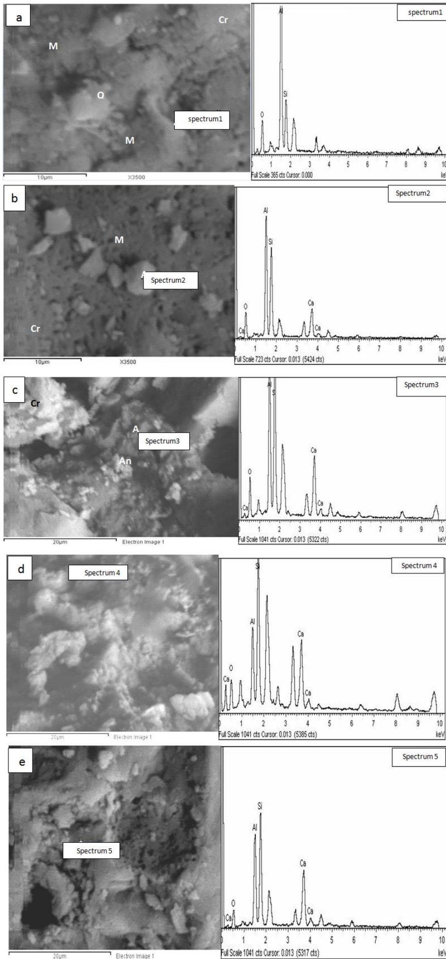
**Figure 4.** (a-e) SEM images with EDX spectra for bodies ( $\gamma$ AS0,  $\gamma$ AS15,  $\gamma$ AS20,  $\gamma$ AS25 and  $\gamma$ AS30, respectively) at vitrified temperature
