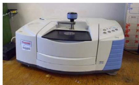
**Figure 6.** Fourier Transform Infrared Spectroscopy (The Thermo Scientific Nicolet iS10)
