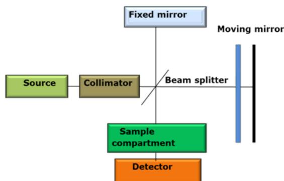
**Figure 3.** Block diagram of an FTIR spectrometer
