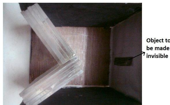
Figure 2. Cross sectional view of the apparatus made of acrylic used to make the object invisible
