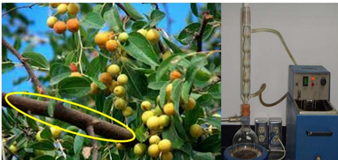
**Figure 1.** *Zizyphus spina Christi*: a) the branches precursor for cellulose isolation, and b) the hydrolysis apparatus used for nanocrystalline cellulose synthesis
