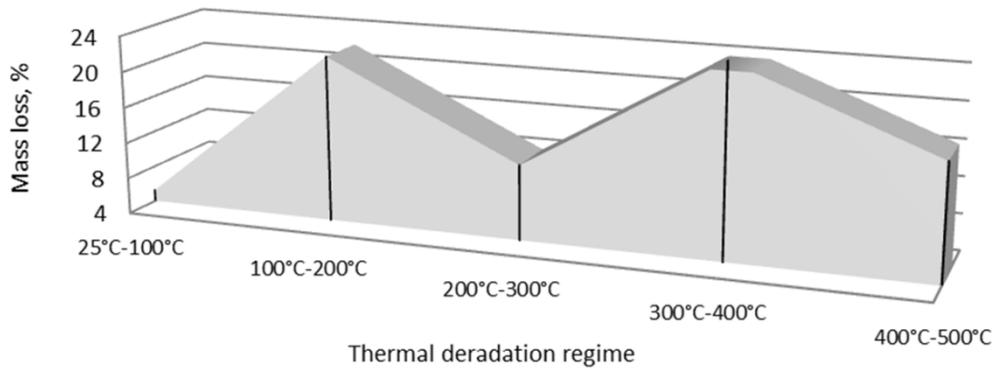
Figure 6. Thermogravimetric analysis (TGA) of the nanocrystalline cellulose (NCCs)
