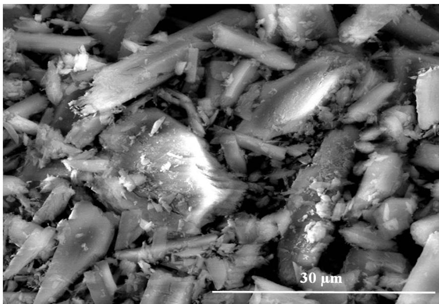
Figure 3. SEM micrograph of agglomerated particles of nanocrystalline cellulose (NCCs) of *Zizyphus spina christi* after oven drying
