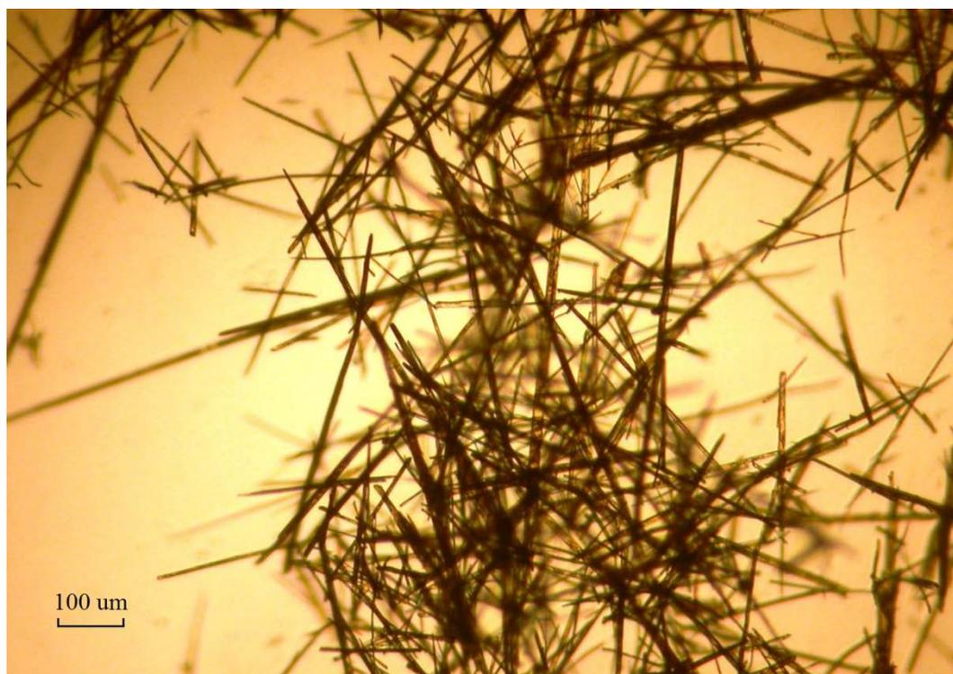
**Figure 2.** An optical image of the needle-shaped nanocrystalline cellulose (NCCs) of *Zizyphus spina christi* directly in an acidic media on a glass substrate
