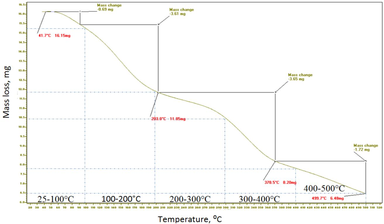
Figure 5. Thermogravimetric analysis (TGA) of the nanocrystalline cellulose (NCCs)
