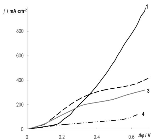
**Figure 4.** Dependence of potential on current density for an oxygen electrode based on  $0.02 \text{ g/cm}^2$  nanostructured composites of nanotubes with deposited molybdenum oxide with an elemental molybdenum content of (wt %): (1) 5.0, (2) 4.0, (3) 3.5, (4) pure carbon nanotubes
