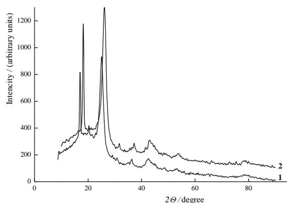
**Figure 3.** X-ray phase analysis of composites sample based on molybdenum oxide and carbon nanotubes containing elemental molybdenum with mass % of: (1) 5.0, (2) 3.5. An apex at  $2\theta=26.04$  degrees corresponds to molybdenum oxide
