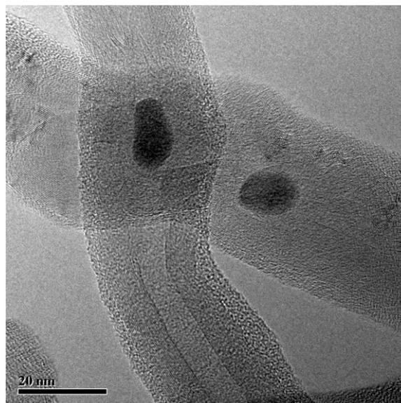
**Figure 2.** Electron micrograph of the sample No 3. Elemental molybdenum content 3.5 wt %
