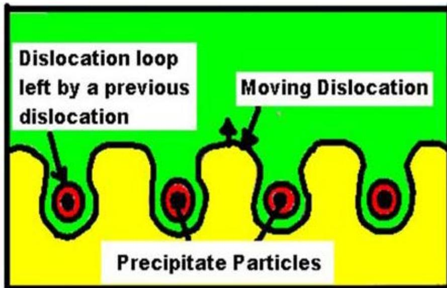
**Figure 2.** Orowan mechanism of strengthening the metal matrix from precipitates (Reprinted from [26])
