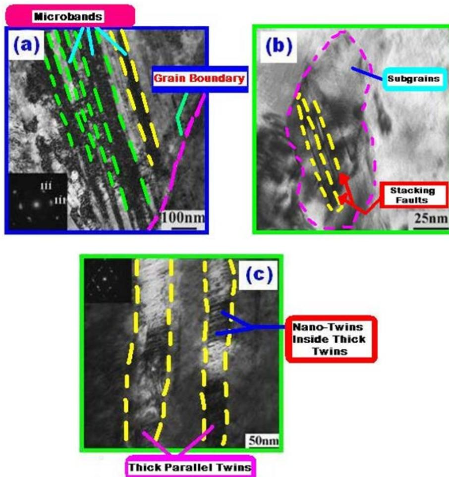
**Figure 8.** TEM Image of (a) Microbands (b) Stacking faults in Subgrain (c) Nano Twins within Thick Twins (Reprinted from [106])
