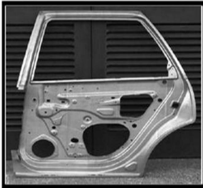
Figure 3. Inner door body panel for automobile from IF steel (Reprinted from [33])
