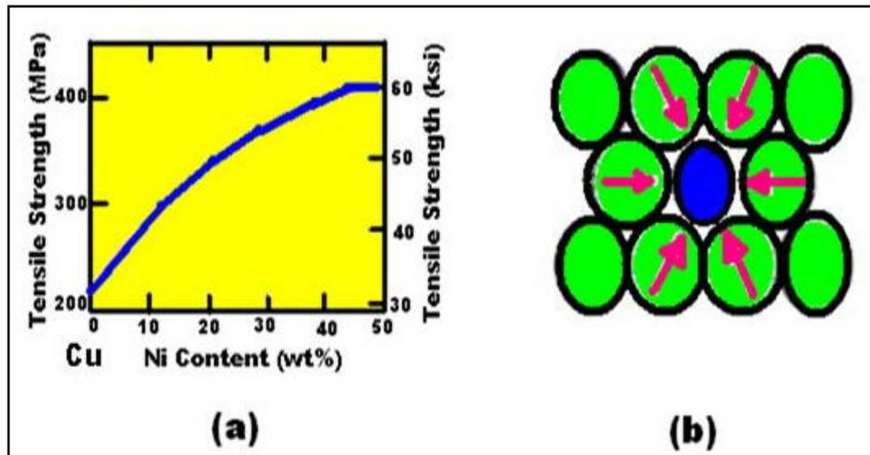
**Figure 1.** (a) Changes of Tensile Strength with increasing Ni content in the Copper- Nickel Alloy (b) Schematic diagram of generation of Lattice strain with incorporation of small substitutional element within the metal (Reprinted from [25])
