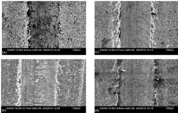
**Figure 5.** SEM scratch test image of AlCrN deposited on (a) EN353/2µm; (b) EN353/4µm; (c) EN31/2µm and (d) EN31/4µm
