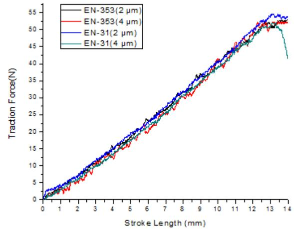
**Figure 4.** Variation of traction force vs stroke length for different coating thicknesses and carbon contents of the substrate.
