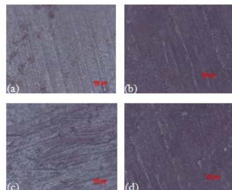
**Figure 1.** Optical microstructure images (100 $\mu\text{m}$ ) of AlCrN coated surfaces of (a) 2  $\mu\text{m}$  on EN353, (b) 4  $\mu\text{m}$  on EN353, (c) 2  $\mu\text{m}$  on EN31 and (d) 4  $\mu\text{m}$  on EN31
