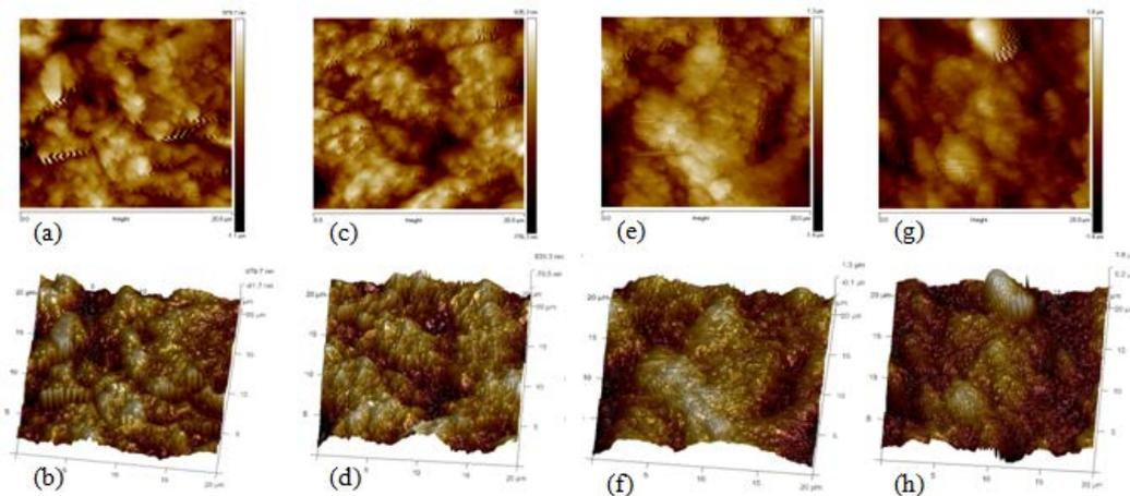
**Figure 2.** 2D and 3D AFM images of AlCrN coating deposited on EN353 (2 $\mu$ m (a, b) & 4 $\mu$ m (e, f)) and EN31 steel (2 $\mu$ m(c, d) & 4 $\mu$ m(g, h)).
