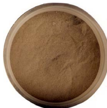
Figure 2. Pulverized Pb-Zn ore
