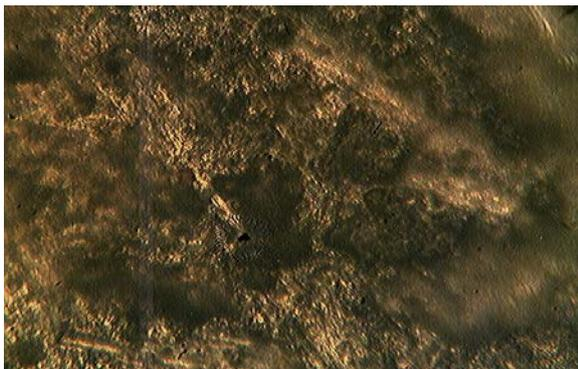
Figure 13. Microstructure of Pb-Sb matrix, 4.76%Cu x400
