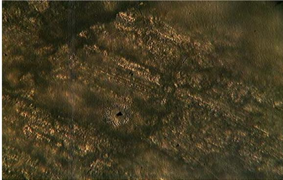
Figure 12. Microstructure of Pb-Sb matrix, 1.96%Cu x400
