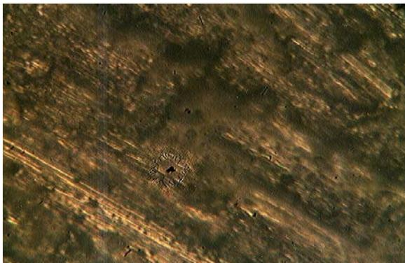
Figure 14. Microstructure of Pb-Sb matrix, 5.66%Cu x400
