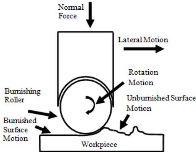
Figure 1. Principle of burnishing tool
