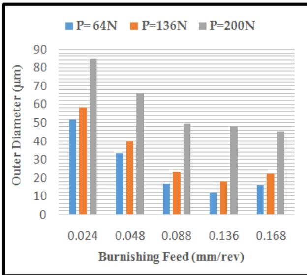
Figure 8. Effect of burnishing feed on roundness error at 48.24m/min burnishing speed
