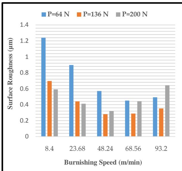
Figure 6. Effect of burnishing speed on surface roughness at 0.088 mm/rev. feed rate
