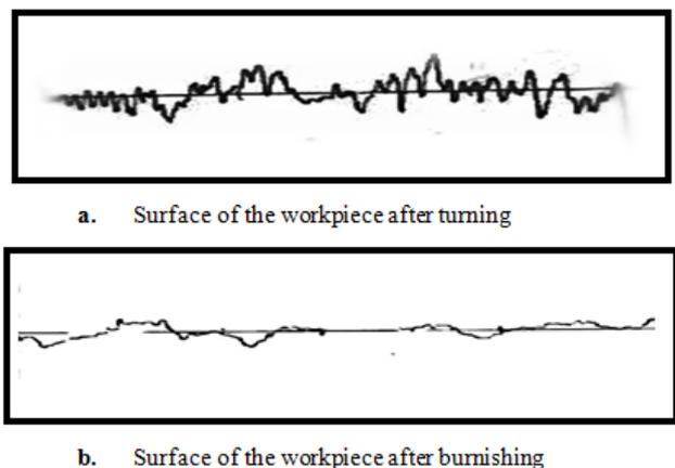
Figure 11. Surface roughness profile before and after burnishing
