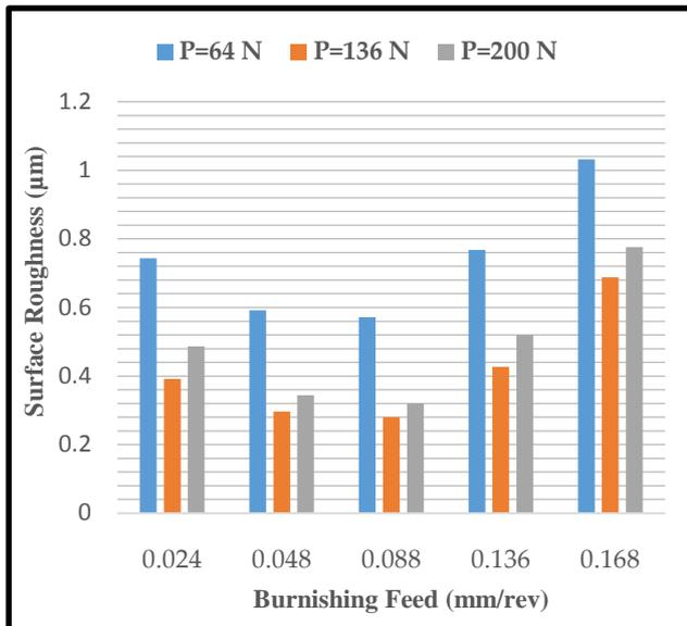
Figure 4. Effect of burnishing feed on surface roughness for different burnishing force
