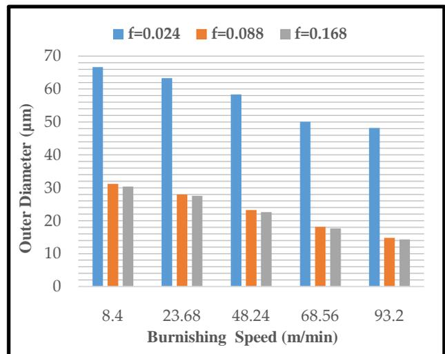
Figure 10. Effect of burnishing speed on roundness error at 136N burnishing force
