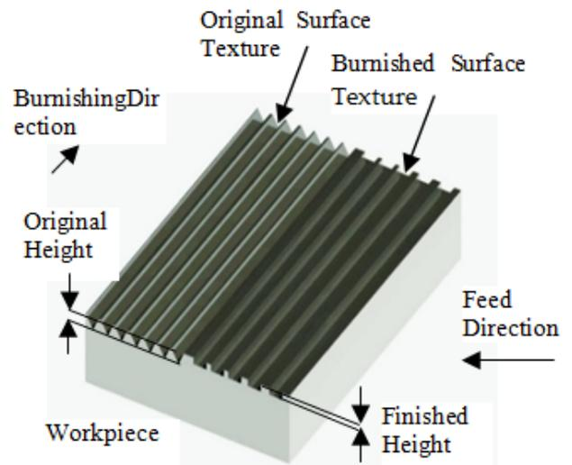
Figure 5. Schematic representation of the burnishing process
