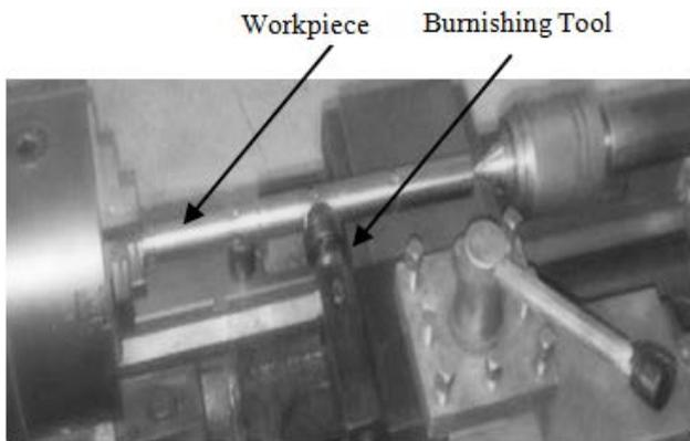
Figure 2. Installation of burnishing tools on a lathe
