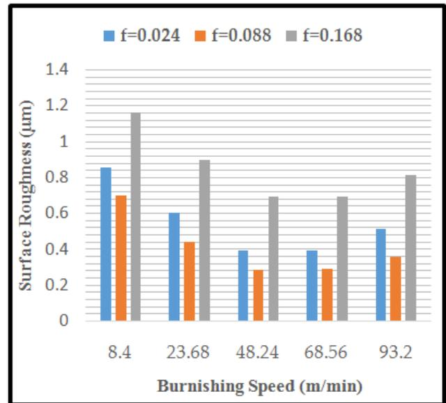
Figure 7. Effect of burnishing speed on surface roughness at 136N burnishing force
