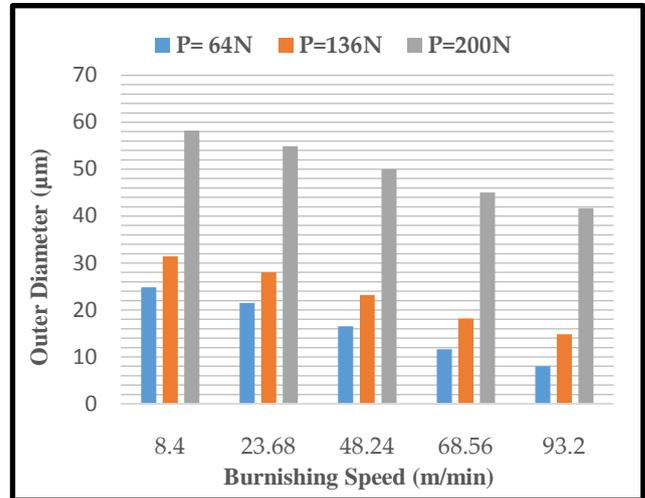
Figure 9. Effect of burnishing speed on roundness error at 0.088mm/rev. feed rate
