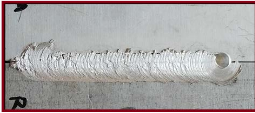
Figure 2. Lateral flash in the joint FSW-A2
