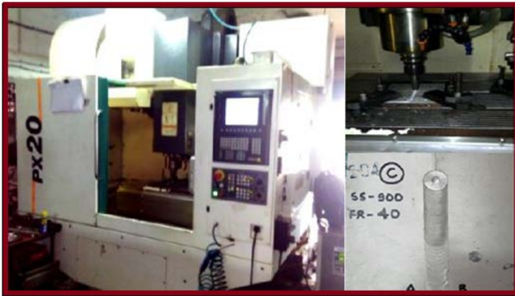
Figure 1. Friction stir welding on VMC machine with FSW joint
