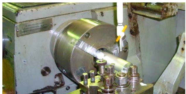
Figure 2. Arrangement for MQL for a feed rate of 0.5 mm/rev
