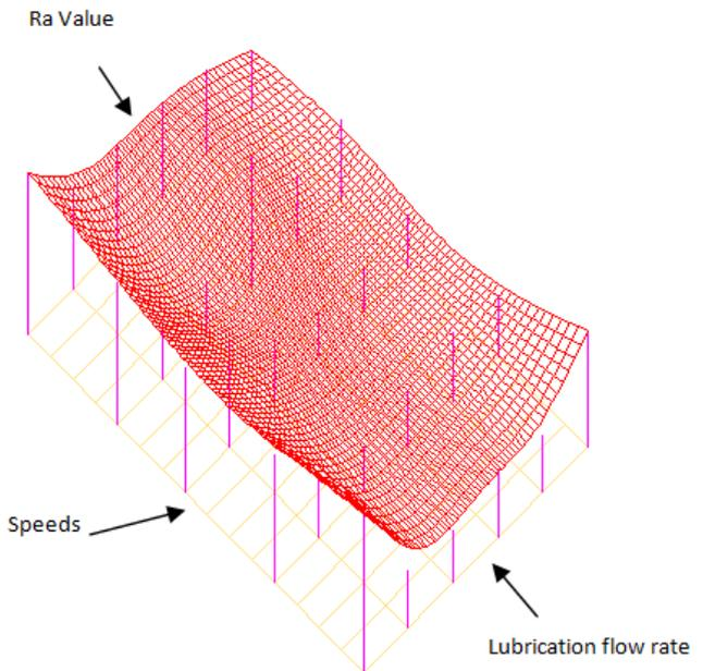
**Figure 11.** Plot of Ra for Feed rate 0.03 mm/rev and Speeds 425--1380
