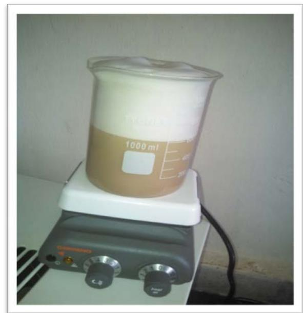
Figure 1. Stirring the mixture with Magnetic stirrer
