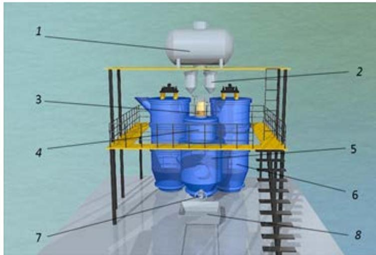
**Figure 1.** Plasma reduction apparatus (PRA - 300): 1 - plasma generator; 2 - reactor - 1 p; 3 - settling chamber, 4 - filters block, 5 - powder feeders; 6 - hopper for raw material; 7 and 7<sup>1</sup> - receiving hopper, consisting of a container and bogey; 10 - auger
