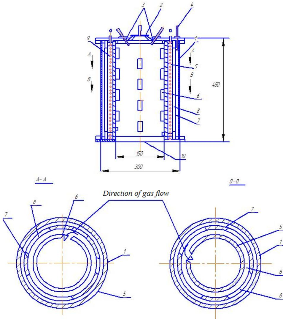
**Figure 2.** Plasma chemical reactor with a high degree of raw material processing: 1 - porous molybdenum cylinder, 2 – porous stainless steel cylinder; 3 - plasmatron A-26 (PG-2, I); 4 - case.
