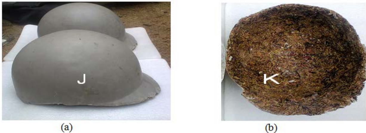
Figure 8. Photographs of cast helmets waiting to be laid with foam liner; (J) External surface of the cast helmet; (K) Internal surface of the cast helmet before and after cleaning off excess materials
