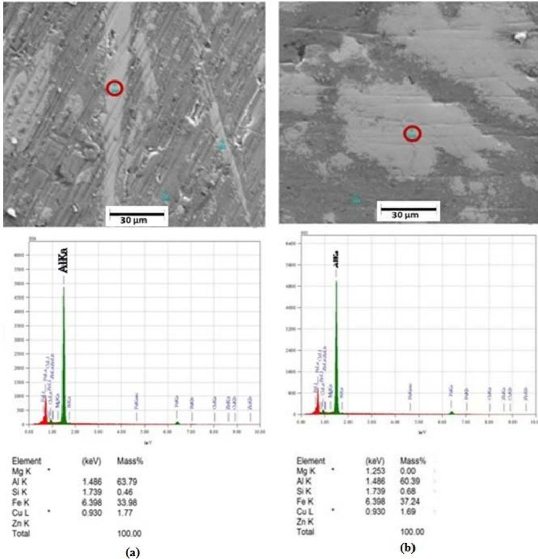
Figure 2. Microstructure [Magnification : 300X] and SEM/EDS spectrum of (a) 2.5 mass% Mg; (b) 4.0 mass% Mg composite
