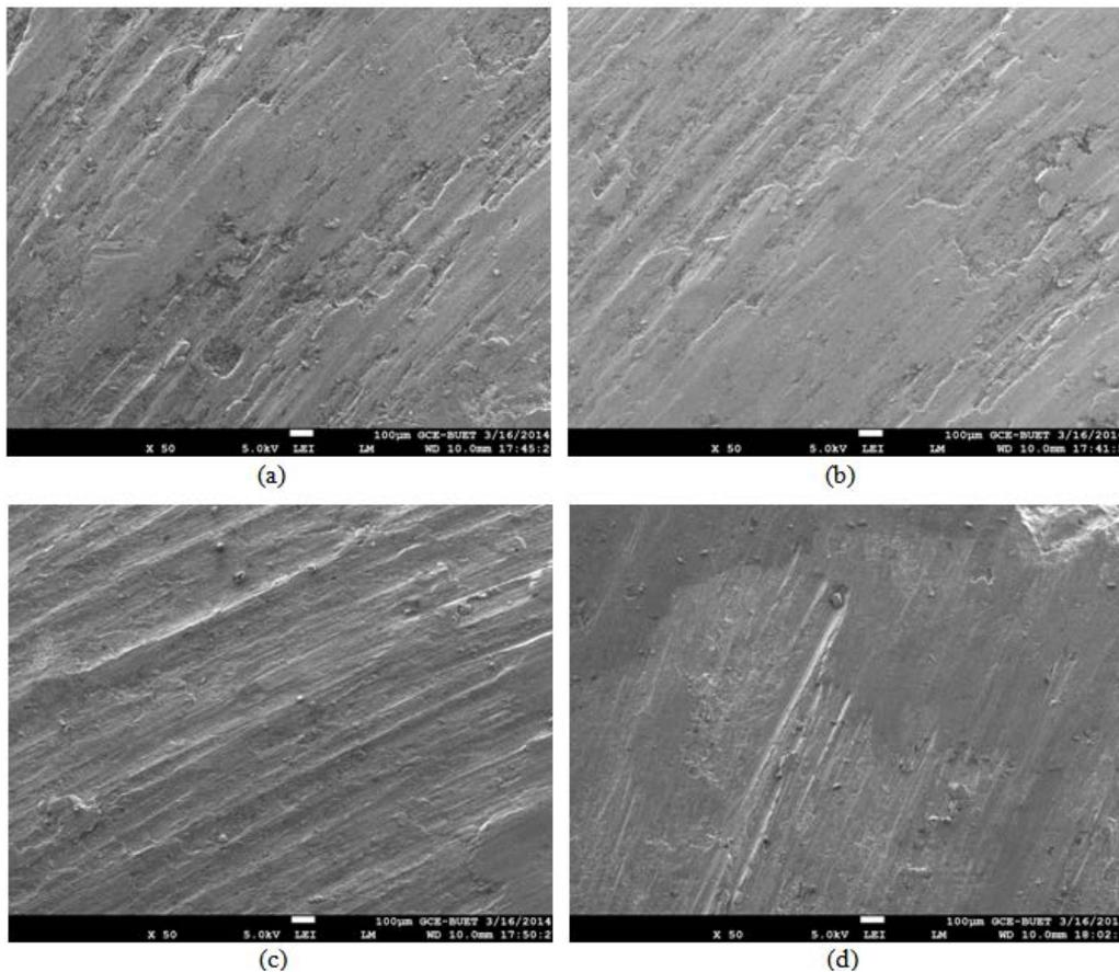
**Figure 5.** Scanning electron micrographs [Magnification : 50X] of the worn surfaces of the composite with (a) 1.5 mass% Mg; (b) 2.5 mass% Mg; (c) 3.5 mass% Mg; (d) 4.0 mass% Mg, subjected to wear test [ load: 15 N; time: 600 seconds
