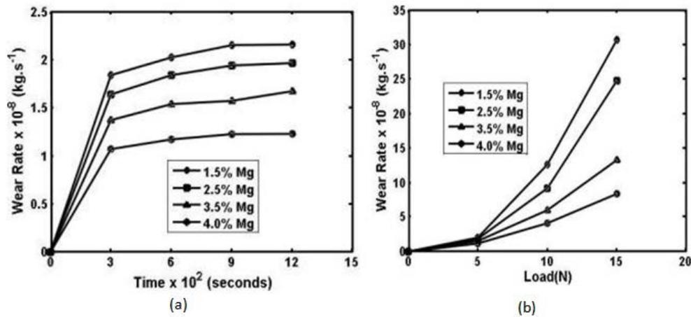
**Figure 3.** Wear rate of as-cast composites with different Mg additions as (a) function of time; (b) function of load
