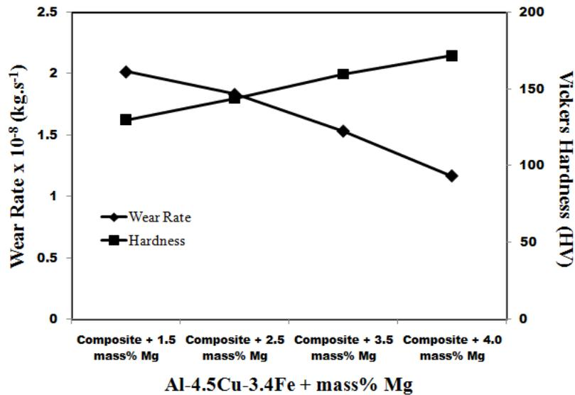
Figure 6. Dependence of Wear Rate and Hardness on Reinforcement
