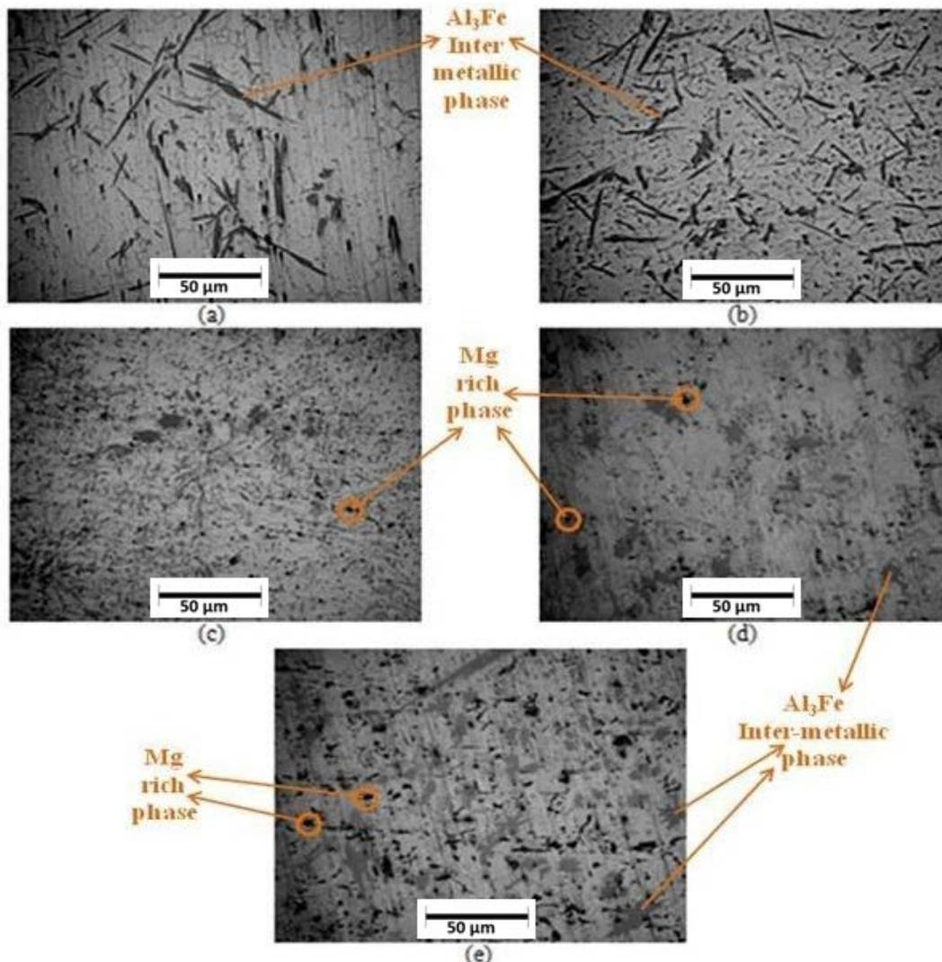
**Figure 1.** Microstructure [Magnification: 200X] of as-cast in-situ composite with (a) no Mg; (b) 1.5 mass% Mg; (c) 2.5 mass% Mg; (d) 3.5 mass% Mg; (e) 4.0 mass% Mg
