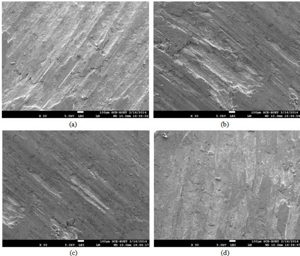
**Figure 4.** Scanning electron micrographs of the worn surfaces of the composite with (a) 1.5 mass% Mg; (b) 2.5 mass% Mg; (c) 3.5 mass% Mg; (d) 4.0 mass% Mg [load 5 N; time: 1200 seconds]
