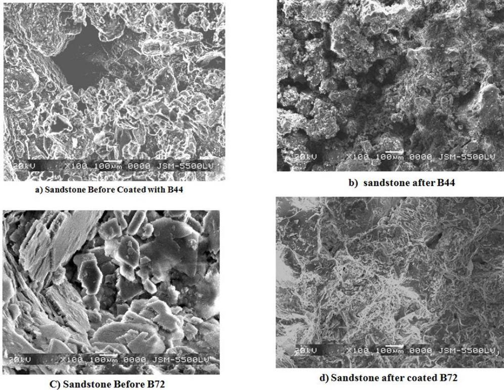
Figure 3. SEM micrograph comparing sandstone after and before coated with B44 and b72
