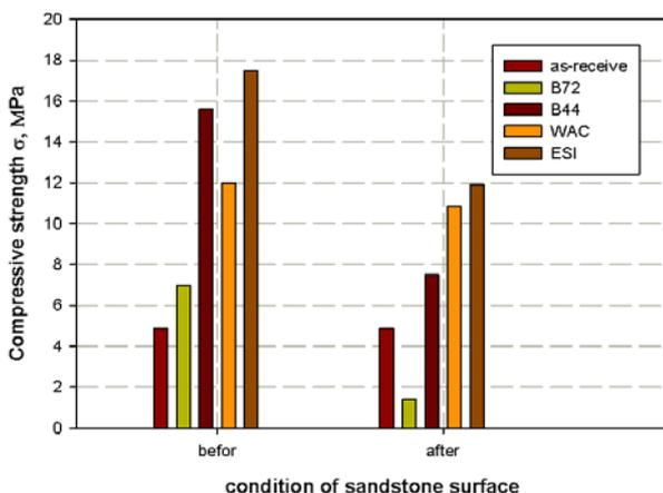
Figure 7. Efficient of coating material for weathering
