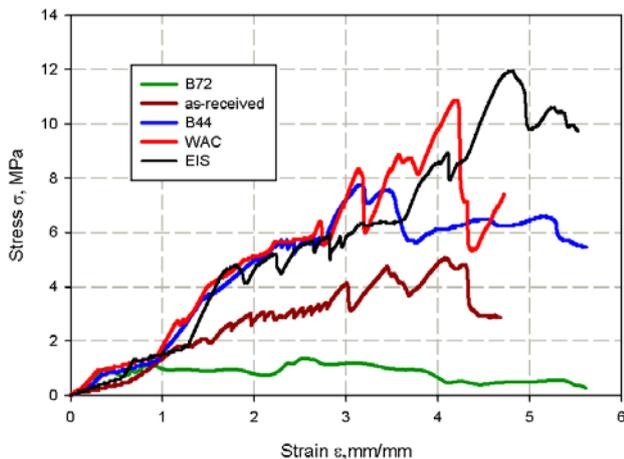
Figure 6. Compressive stress strain diagram for various coating materials after immersed in water
