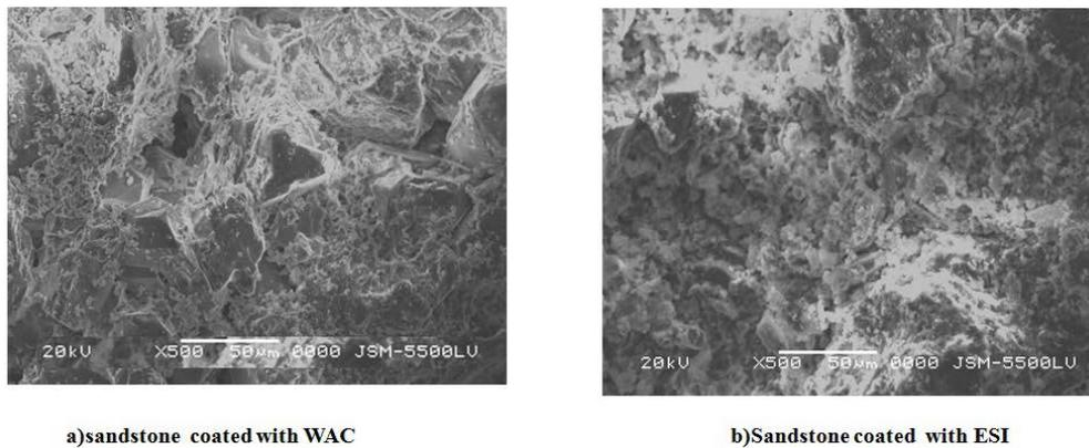
Figure 4. SEM micrograph comparing sandstone after and before coated with ESI and WAC
