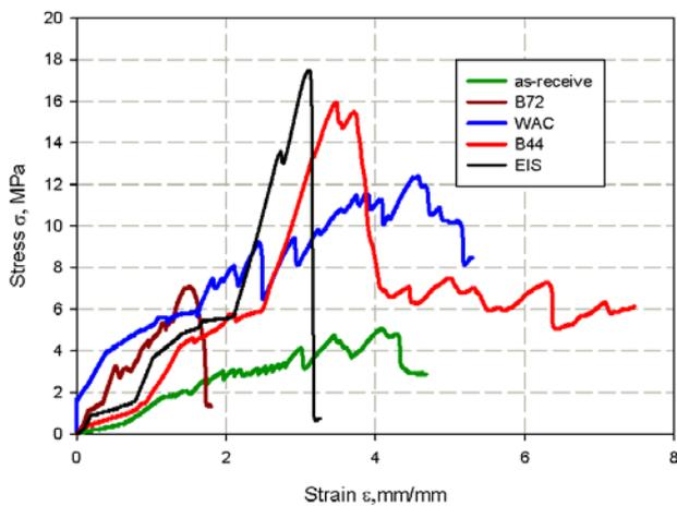
Figure 5. Compressive stress strain diagram of different coating materials
