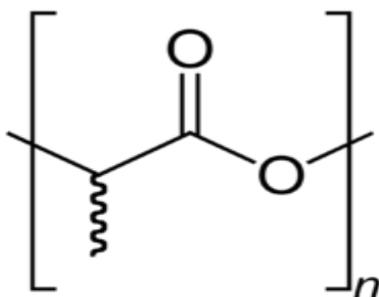
Figure 1. Chemical structure of Poly(lactic acid)
