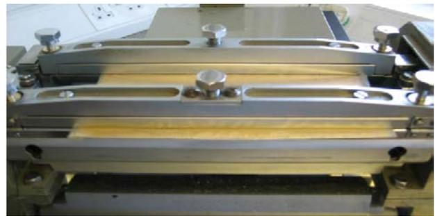
Figure 6. KES- FB Shear Tester [MODEL KES-FB1]
