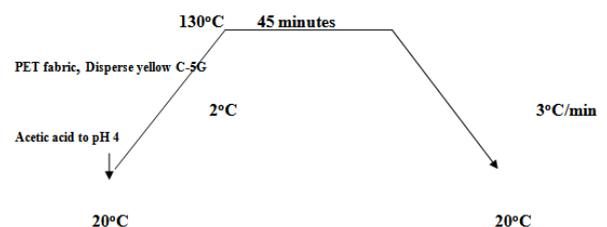
**Figure 4.** Procedure of disperse dye applied to PET
