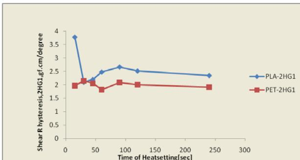
Figure 10. Effects of time of heatsetting and wet treatments on Shear Hysteresis 2HG<sub>1</sub> of Knitted PLA and PET
