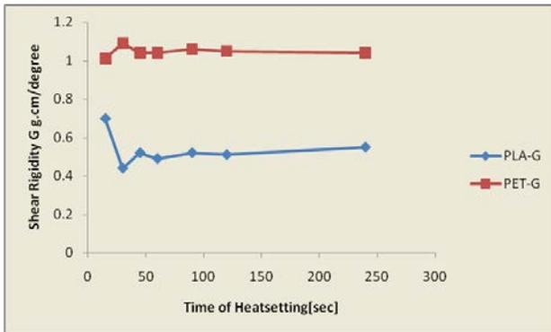
Figure 9. Mean Effects of increasing time of Heatsetting on mean shear rigidity G of Knitted PLA and PET
