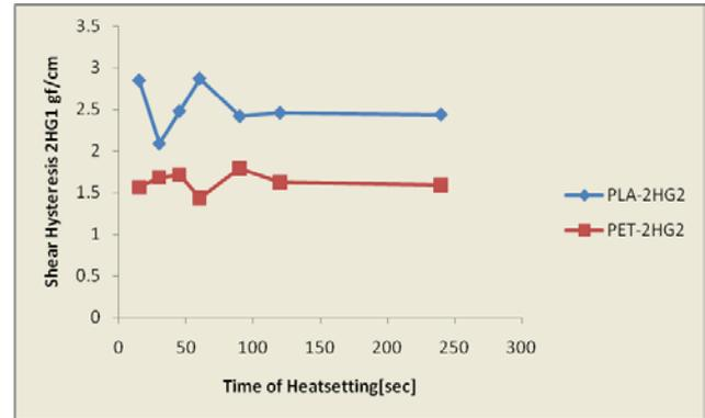
Figure 11. Effect of increasing time of heatsetting and wet treatments on Shear Hysteresis 2HG<sub>2</sub> on knitted PLA and PET
