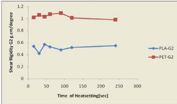
Figure 8. Effects of increasing time of Heatsetting and wet processing on Shear Rigidity  $G_2$  gf.cm/degree of knitted PLA and PET
