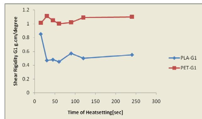
Figure 7. Effects of increasing time of Heatsetting and wet processing on Shear Rigidity G<sub>1</sub>, gf.cm/degree of knitted PLA and PET
