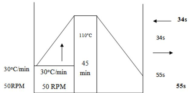
**Figure 3.** Mathis LABOMAT Uniprogrammer PLA dyeing procedure
