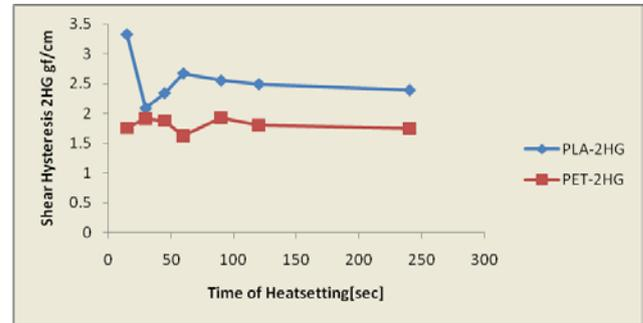
Figure 12. Effect of time of heatsetting and wet treatment on mean of Shear Hysteresis [2HG] of knitted PLA and PET
