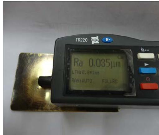
Figure 5. Surface roughness tester, (TR-220)
