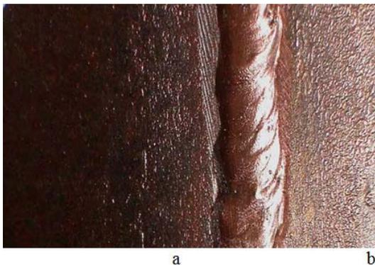
Figure 2. Welding copper to steel using a pulsed preheating, a-steel; b-copper
