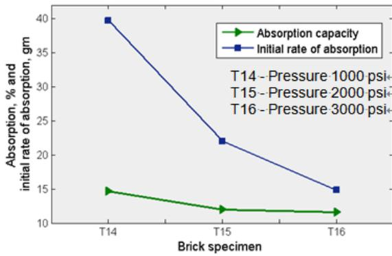
Figure 9. Effect of brick forming pressure on absorption capacity and IRA
