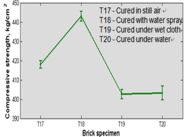
Figure 12. Effect of curing process on compressive strength
