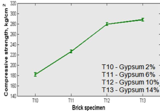
Figure 5. Effect of gypsum addition on compressive strength
