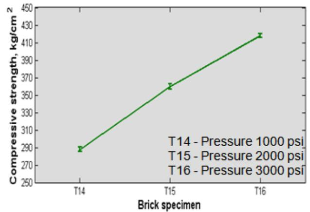
Figure 6. Effect of brick forming pressure on compressive strength
