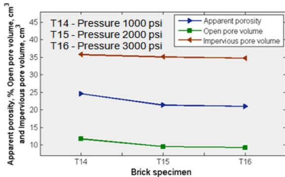
Figure 10. Effect of brick forming pressure on apparent porosity, open pore and impervious pore volume
