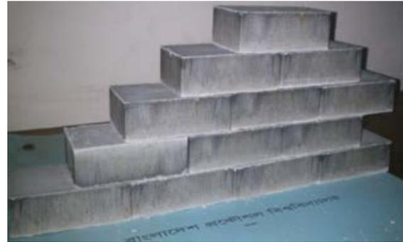
**Figure 2.** Fly ash-sand-lime-gypsum bricks
