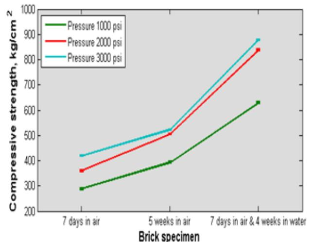
Figure 13. Effect of curing process on compressive strength
