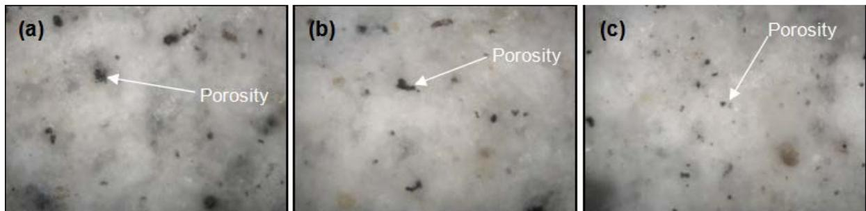
Figure 7. Microstructure of bricks formed with pressure (a) 1000 psi (b) 2000 psi (c) 3000 psi [All magnification 500X]
