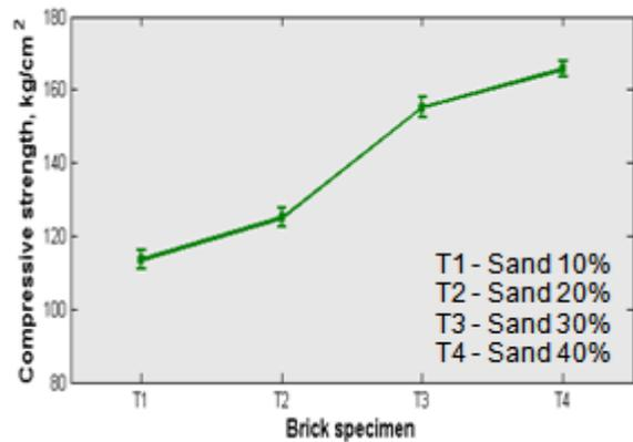
Figure 3. Effect of sand addition on compressive strength
