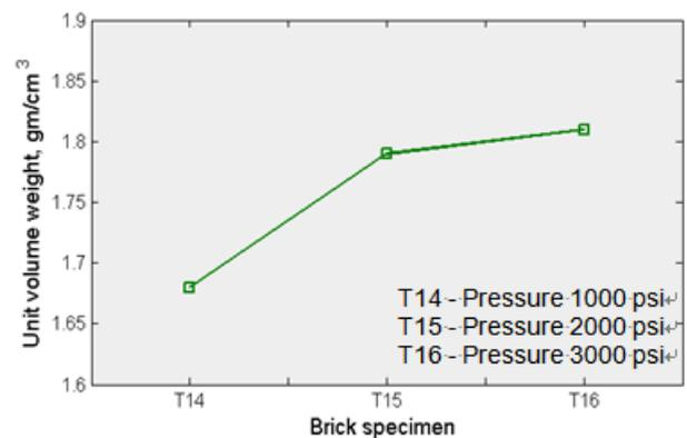
Figure 8. Effect of brick forming pressure on unit volume weight
