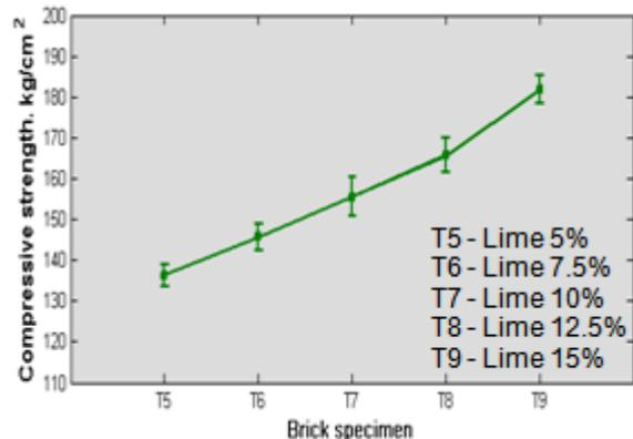
Figure 4. Effect of lime addition on compressive strength
