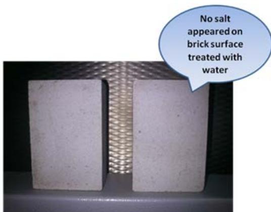
Figure 11. Efflorescence test of bricks of optimum composition
