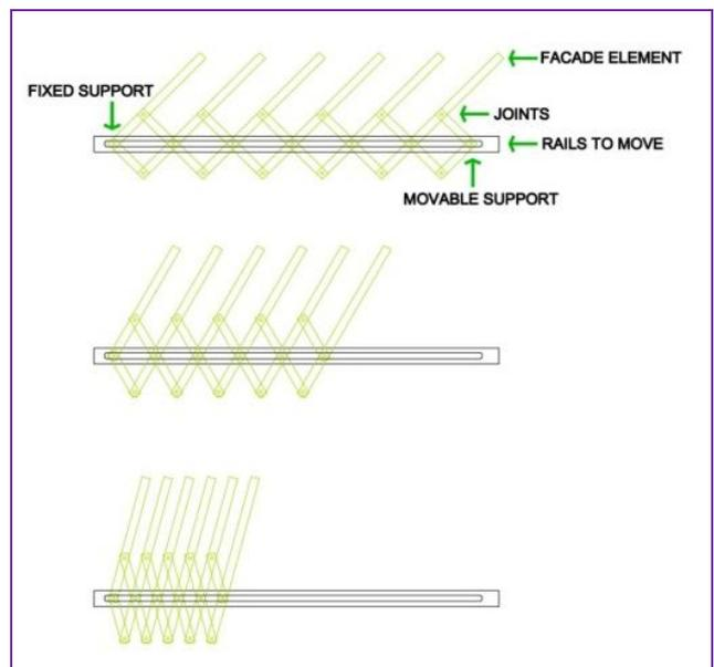
Figure 9. Model of movement phases of idea No. 2
