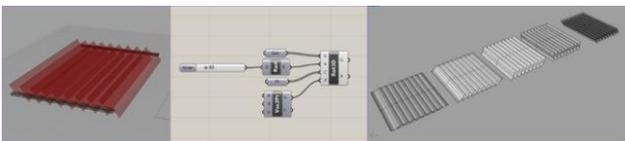
Figure 7. Modeling the movement phases by Grasshopper software and presenting the various movement phases of this idea
