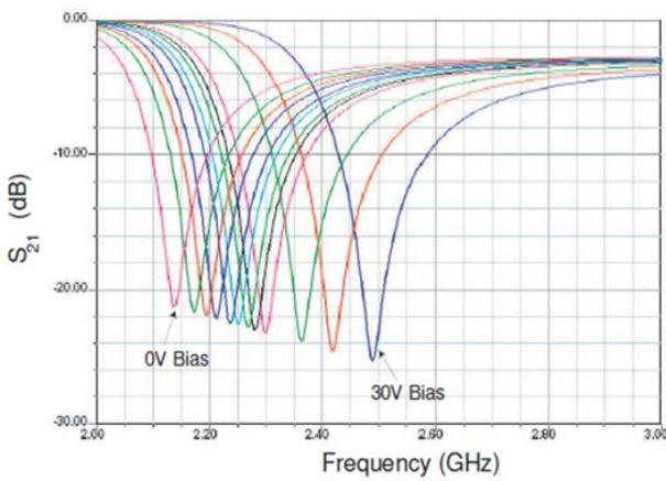
Figure 16. Characteristic response with different applied voltages
