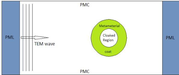
Figure 2. Computational domain and details for the full-wave cloaking simulation
