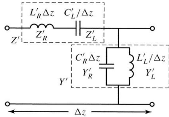
Figure 13. Resonant Circuit for CRLH material
