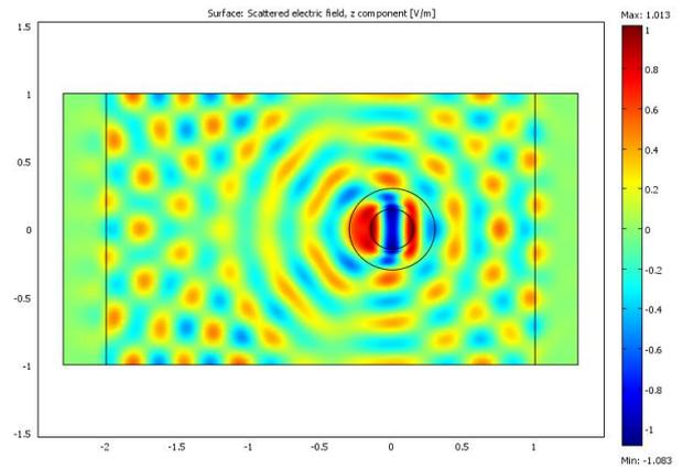
Figure 5. Scattering electric field inside metamaterial
