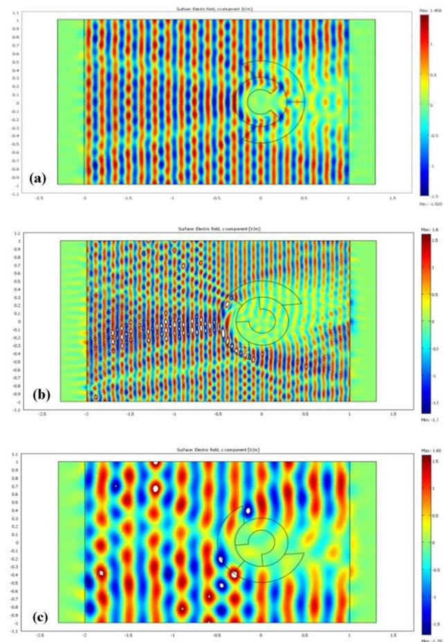
Figure 11. Electric field. Up-Down: 2GHz, 3GHz, 1GHz
