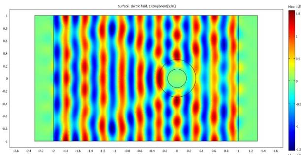
Figure 4. Electric field behavior with metamaterial cloak
