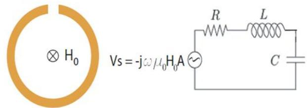
Figure 14. Split Ring Resonator and its equivalent circuit
