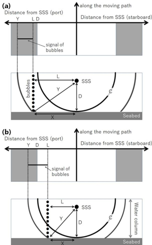
**Figure 3.** Schematic drawing of the relation between sonograph and vertical section of sea (a) when  $L > D$  and (b) when  $L < D$ , where  $L$  is the distance between SSS and the bubble plume and  $D$  is the altitude of SSS
