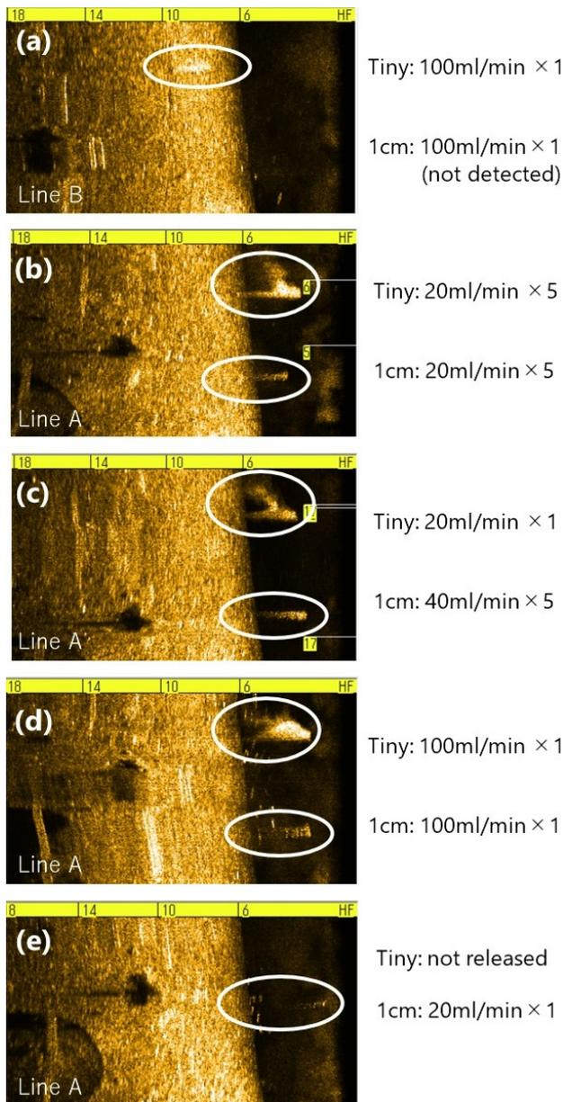
**Figure 4.** Examples of sonograph observed along Line A (b-e) and Line B (a) at a speed of 2 knots
