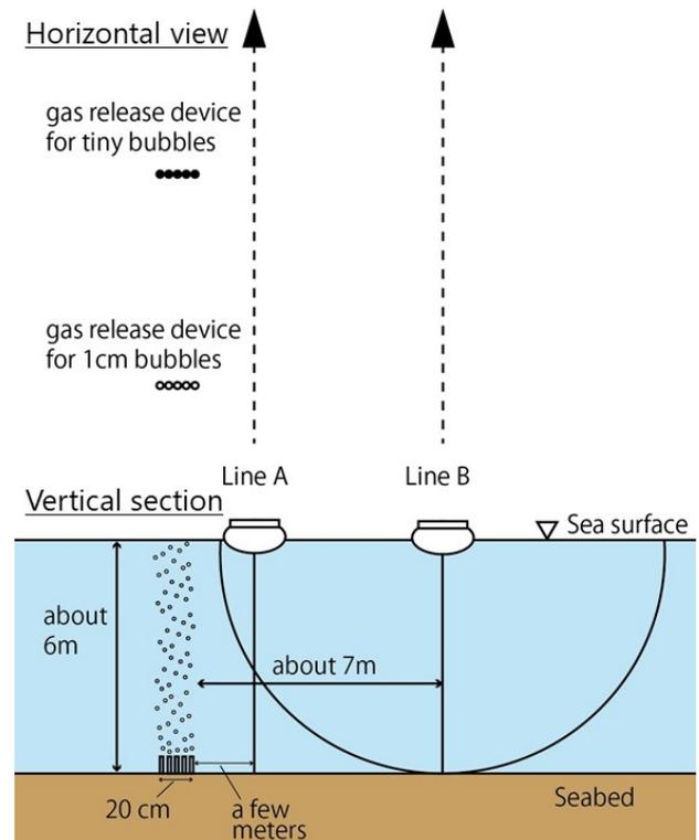
**Figure 2.** Schematic drawing of the positional relation between observation lines and gas release devices
