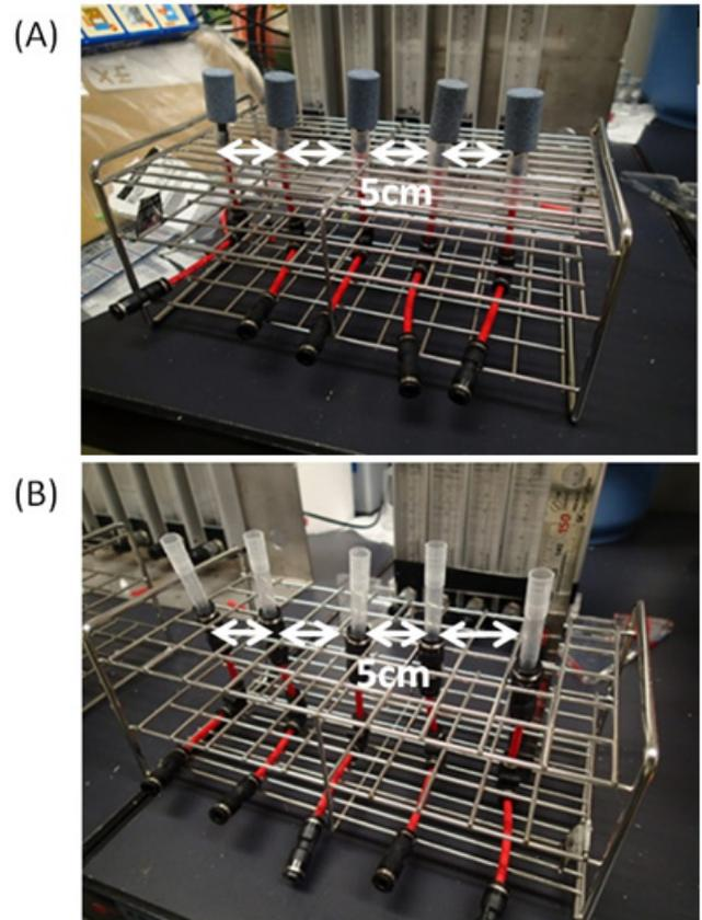
**Figure 1.** Gas release devices with five outlets arranged at intervals of 5 cm for tiny bubbles (A) and 1 cm bubbles (B)
