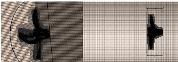
Figure 2. Meshing of the domain and propeller
