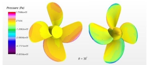
Figure 10. Pressure contour on the propeller surface at J=0.5 and flow angle of 30°
