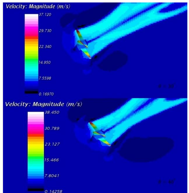
Figure 9. Velocity contour around the propeller at J=0.29 and flow angle of 30° and 40°
