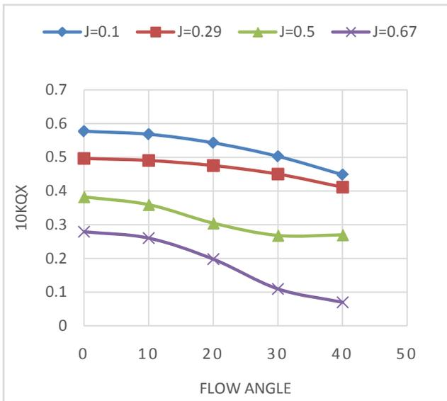
Figure 6. Torque coefficient against flow angle
