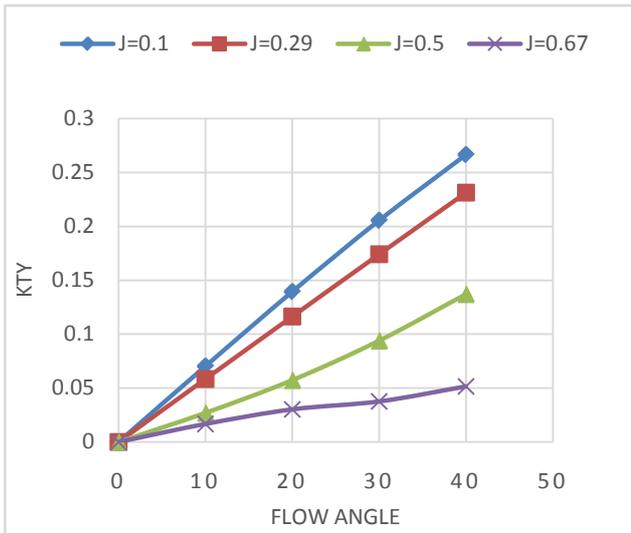
Figure 5. Lateral force coefficient against flow angle
