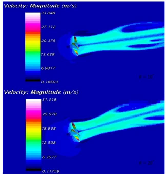
Figure 8. Velocity contour around the propeller at J=0.29 and flow angle of 10° and 20°
