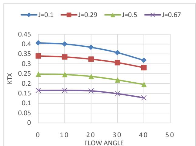
Figure 4. Thrust coefficient against flow angle
