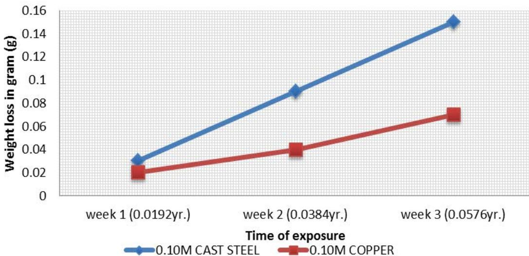
Figure 8. Weight Loss versus Exposure Time of Cast Steel and Copper in 0.1M of Sea Water
