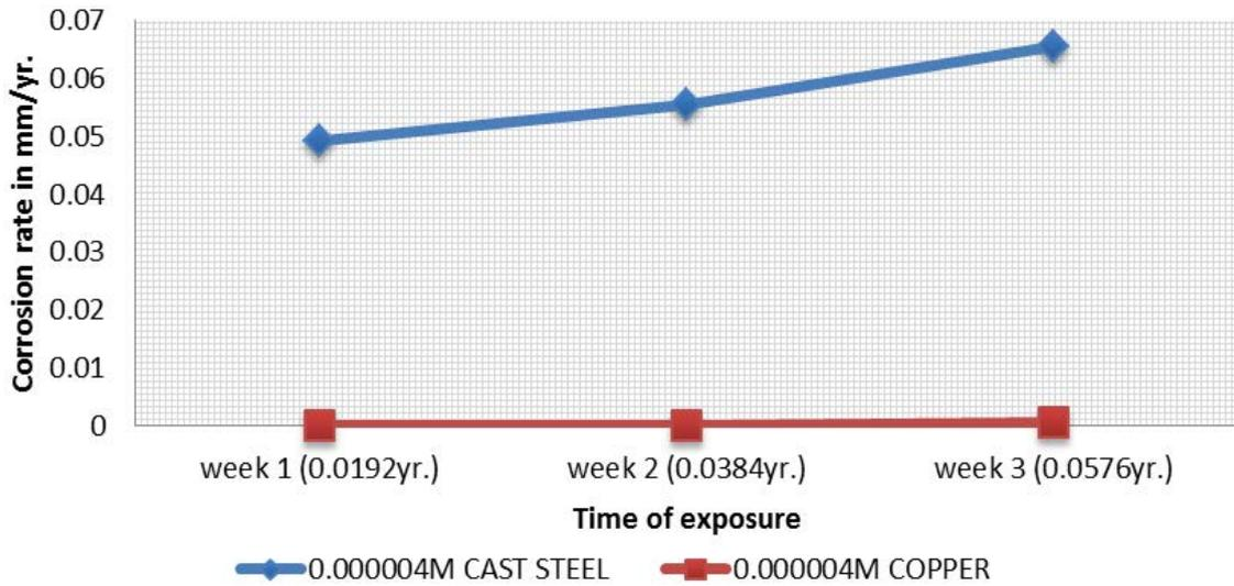
Figure 6. Corrosion Rate versus Time of Exposure of Cast Steel and Copper in 0.000004M of Freshwater
