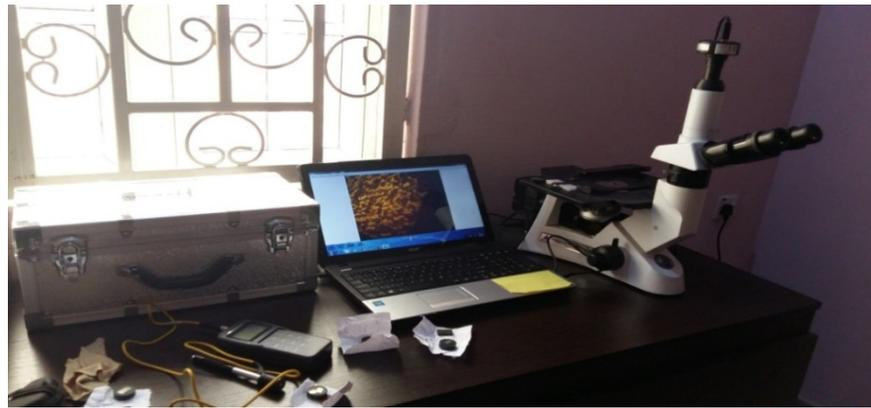
Figure 5. Experimental set up for scanning of the specimens using the Inverted Metallurgical Microscope
