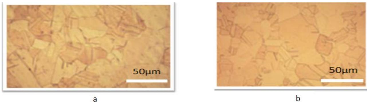
**Figure 12.** a: Micrographs of Copper before Immersion, 12b: Micrograph of Copper after Immersion
