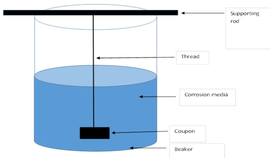
**Figure 2.** Beaker used for corrosion medium
