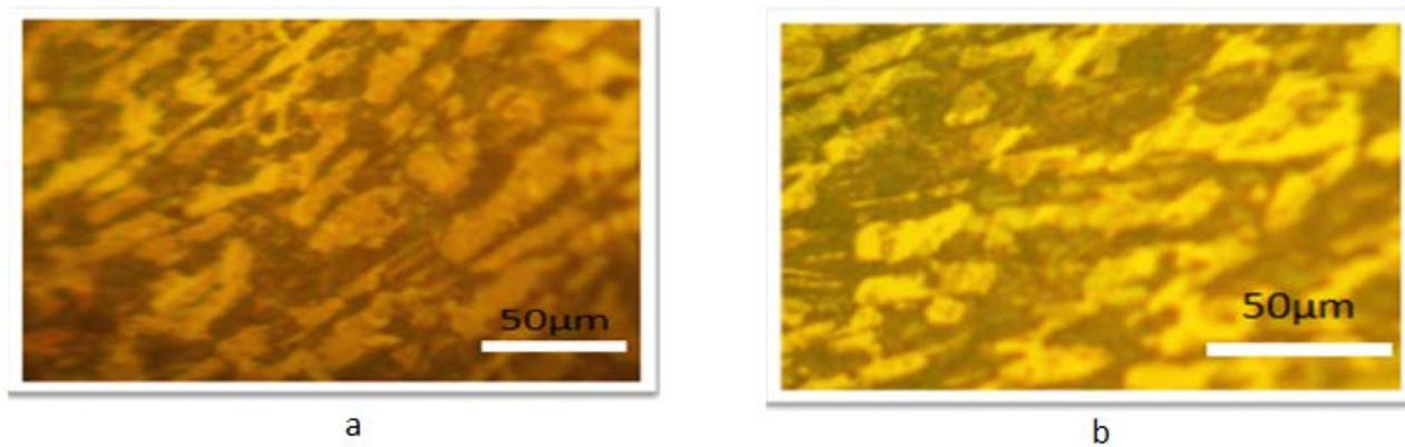
**Figure 11.** a: Micrographs of cast Steel before Immersion, b: Micrographs Cast Steel after Immersion
