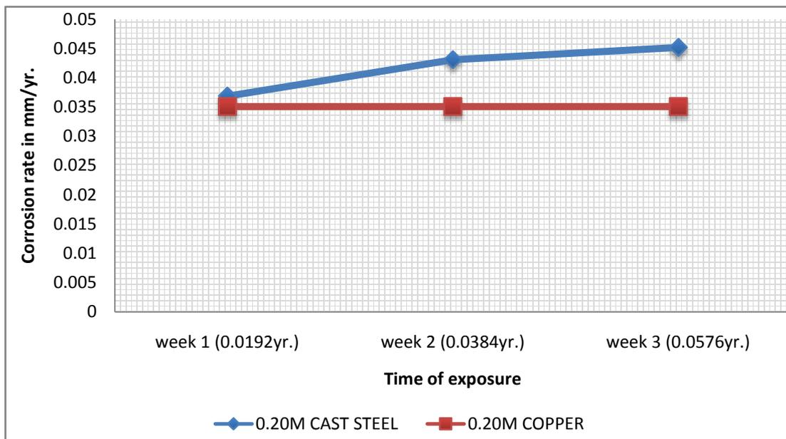
Figure 10. Corrosion Rate versus Exposure Time of Cast Steel and Copper in 0.20M of Seawater
