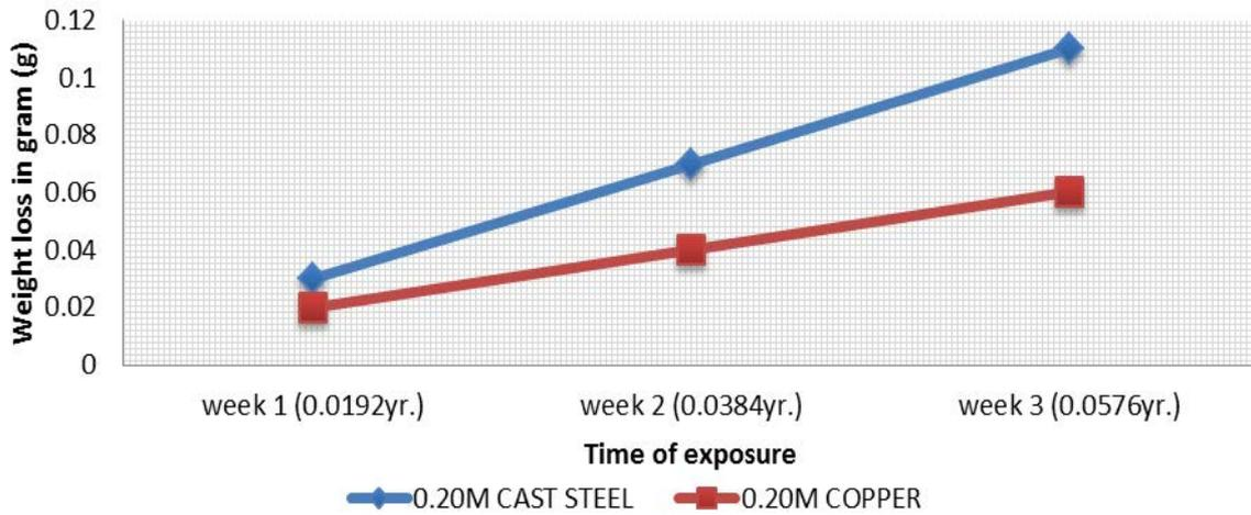
Figure 9. Weight Loss versus Exposure Time of Cast Steel and Copper in 0.000004M of Freshwater
