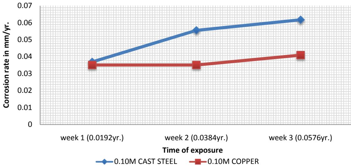
Figure 7. Corrosion Rate versus Exposure Time of Cast Steel and Copper in 0.1M of Sea Water
