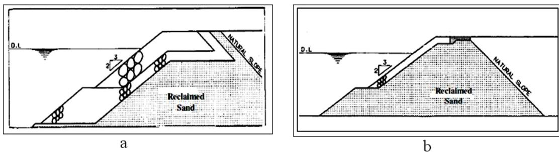
Figure 5. (a) and (b) are typical sea wall and light protection sections for dredged materials usage
