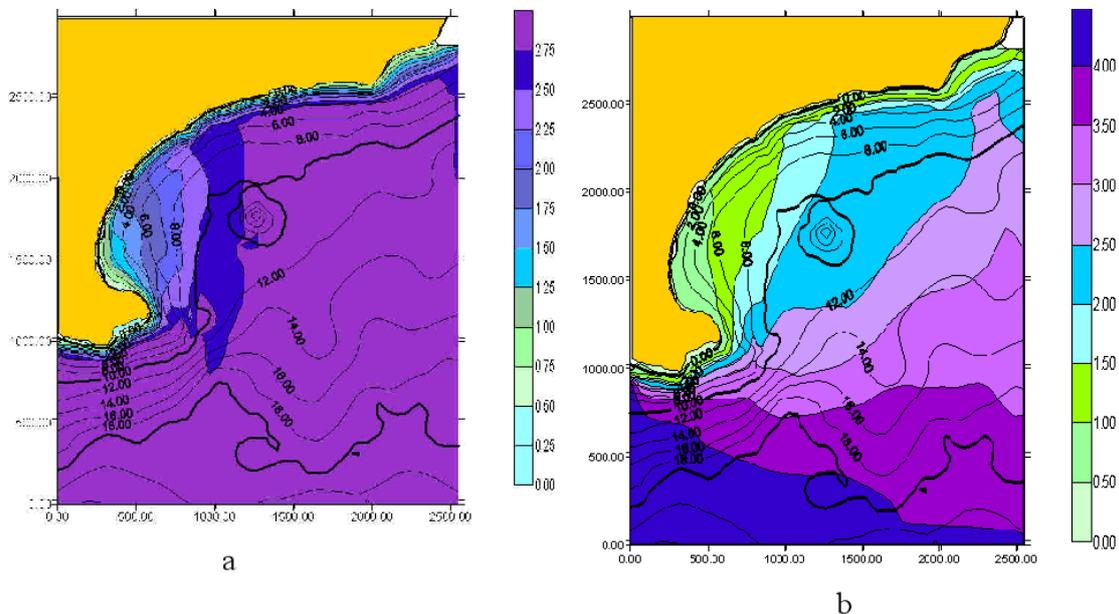
**Figure 1.** (a) Waves nearshore transformation for swell ( $H_s$  (1/1 year)<sub>Swell</sub> = 3.40 m,  $T_p$  = 13 Sec. and propagation direction from  $180^\circ$  to north) and (b) wind sea waves ( $H_s$  (1/1 year)<sub>Wind Sea</sub> = 4.50 m,  $T_p$  = 7.60 Sec. and propagation direction from  $245^\circ$  to north), respectively
