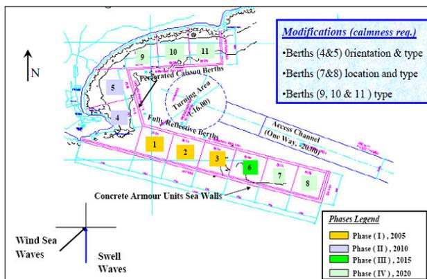
**Figure 2.** Development phases for the open basin and port in a bay facing accretion accumulated on its southern boundary. Phase (I): Berths Number (1, 2 and 3), Phase (II): Berths Number (4 and 5), Phase (III): Berths Number (6) and Phase (IV): Berths Number (7 through 11), respectively
