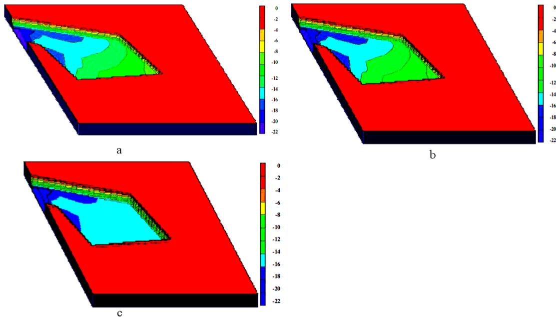
Figure 4. (a), (b) and (c) are soil levels within the port basin area for both conditions Before and after dredging to the design levels
