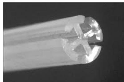
**Figure 4.** Tip of the drain with its flutes
