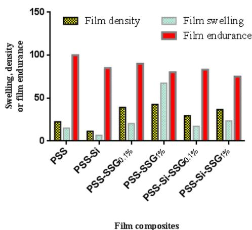
**Figure 4.** Densities ( $\rho_{\text{film}} \times 10^{-3} \text{ g cm}^{-3}$ ), swellings (S) and folding endurance (folds) of PSS film and its composites
