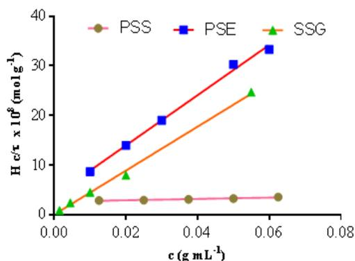
**Figure 2.** A plot of  $Hc/\tau$  versus the concentration of PSS, PSE, and SSG polymers ( $R^2$  for PSS = 0.9496, for PSE  $R^2=0.9951$ , and for SSG  $R^2=0.9970$ )
