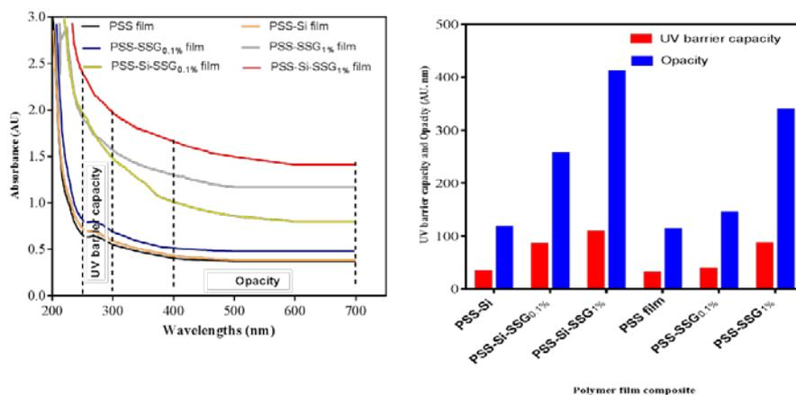
**Figure 3.** Absorption spectra, opacity (blue bars), and UV-barrier capacity (red bars) of potato starch soluble film (PSS), PSS with silica film (PSS-Si), PSS with 0.1 % of starch glycolate film (PSS-SSG0.1%), PSS with 1 % of starch glycolate film (PSS-SSG1%), PSS with silica and 0.1 % of starch glycolate film (PSS-Si-SSG0.1%), and PSS with silica and 1 % of starch glycolate film (PSS-Si-SSG1%)
