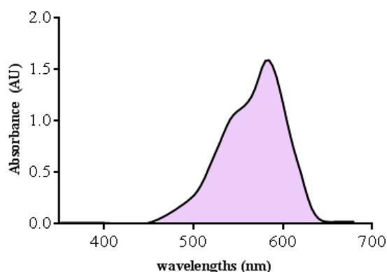
**Figure 6.** UV-vis absorption scan in a range equal to 350-650 nm for crystal violet ( $12.5 \mu\text{M}$  in chloroform) at  $37^\circ\text{C}$
