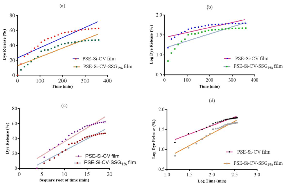
**Figure 8.** Zero order (a), first order (b), Higuchi model (c), and Korsmeyer-Peppas model (d) kinetics release of CV from PSE-Si-CV and PSE-Si-CV-SSG<sub>1%</sub> films in phosphate buffer solution (PBS) pH 7.4 at 37°C
