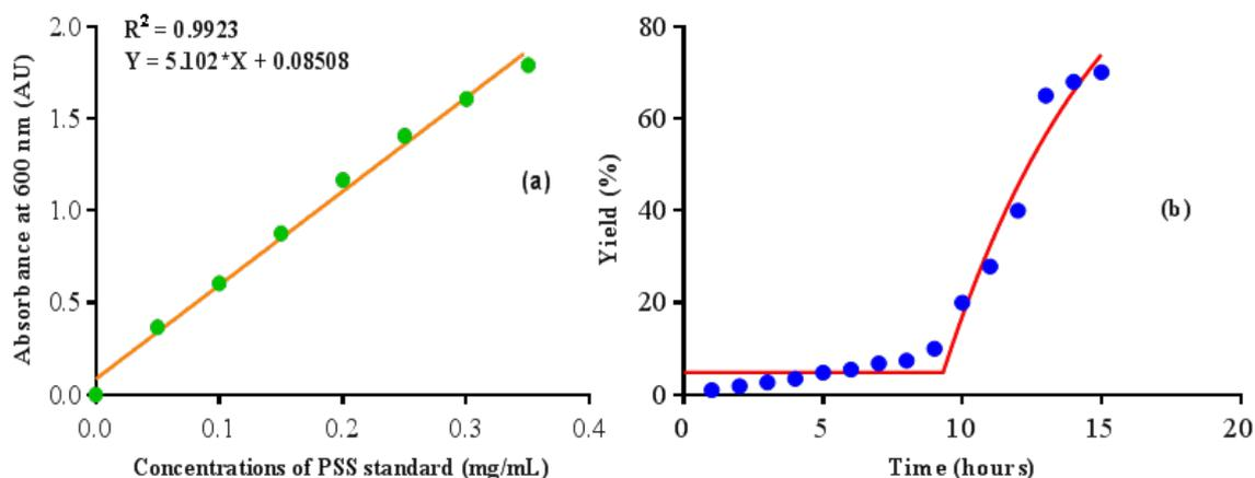
**Figure 1.** Standard curve for PSS solutions using absorbance at 600 nm (a). Kinetics for experimental data of starch yield per one gram of potato (dots) a combined with a mathematical fitting, plateau followed by one phase decay (solid lines)
