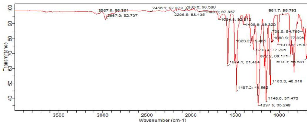
Figure 5. FTIR spectrum of pure MAE/PS compositions
