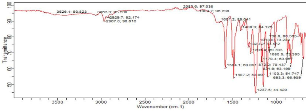
Figure 6. FTIR spectrum of 5% MAE / PS compositions
