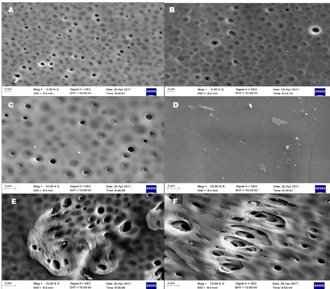
Figure 8. SEM Micrograph of the Active PS Films (A: Pure 0% MAE, B: 1% MAE, C: 2.5% MAE, D: 5% MAE, E: 5% blend of MAE/AT, F: 5% AT)
