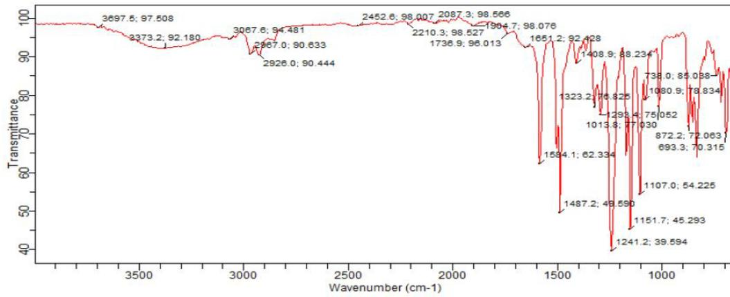
Figure 7. FTIR spectrum of 5% MAE/AT PS blend
