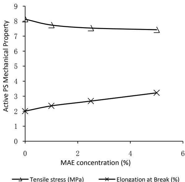
Figure 1. PS mechanical properties vs MAE concentration from 0 - 5%
