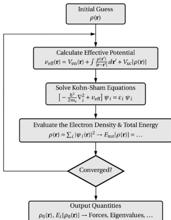
Figure 1. The iteration scheme in the DFT calculation
