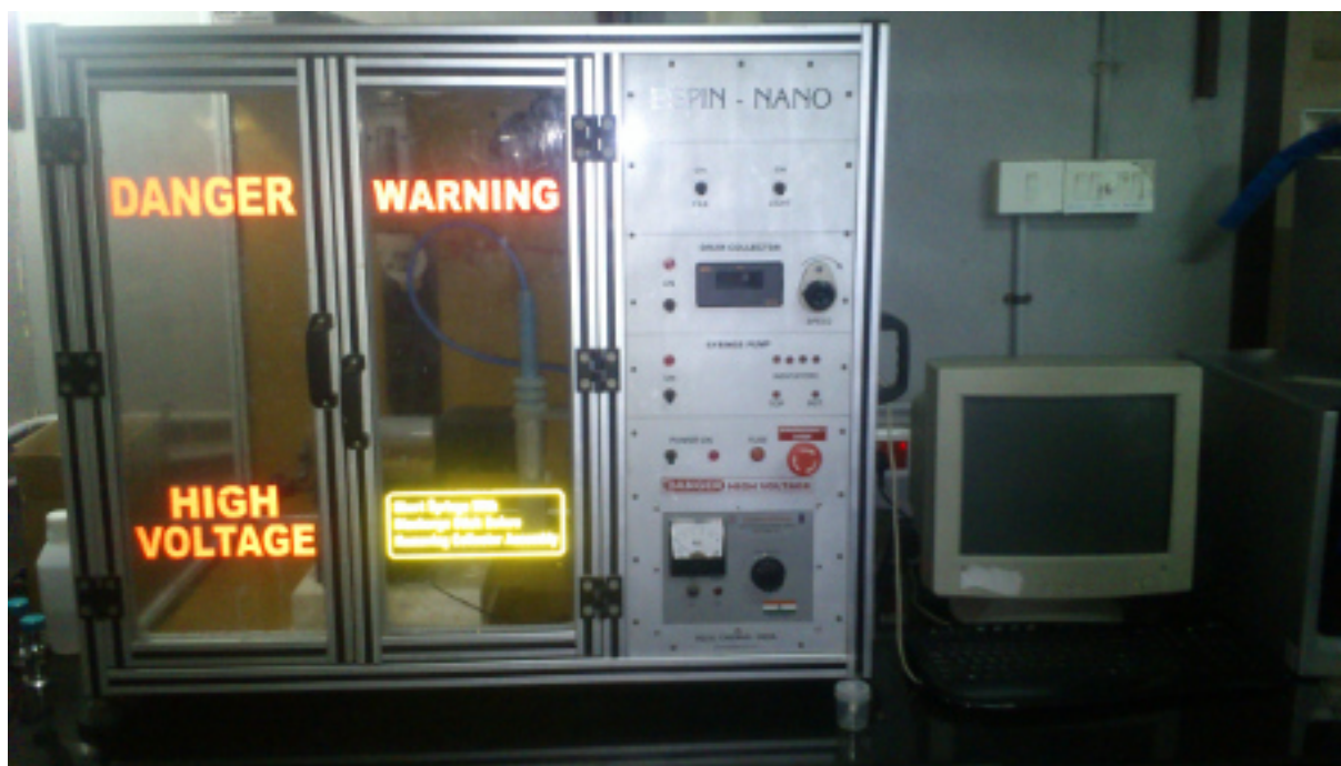
Figure 2. Electrospinning machine used for present study
