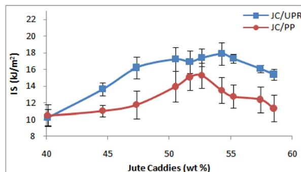
**Figure 4.** Impact strength of JC/UPR and JC/PP composites against fibre loading
