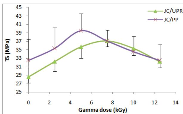
Figure 5. Tensile strength of irradiated JC/ UPR and JC/PP composites (50 wt% fibre)
