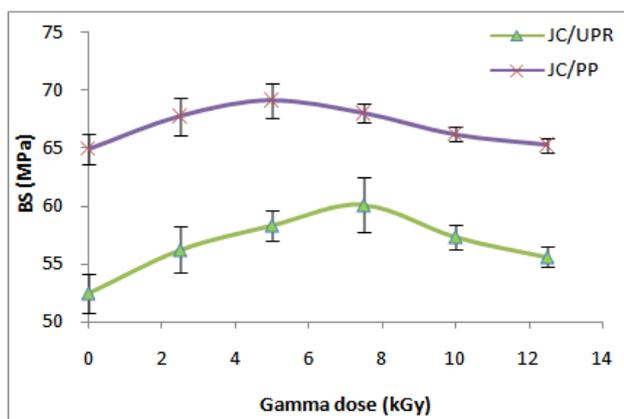
Figure 6. Bending strength of irradiated JC/ UPR and JC/PP composites (50 wt% fibre)
