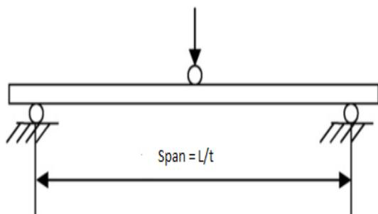
Figure 1. Flexural test configuration
