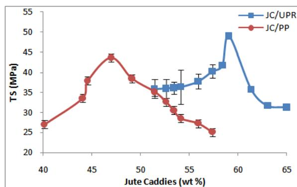
**Figure 2.** Tensile strength of JC/UPR and JC/PP composites with fibre loading
