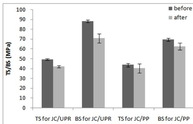
**Figure 8.** Tensile and bending strength of composites (50 wt% fibre) before and after soil degradation
