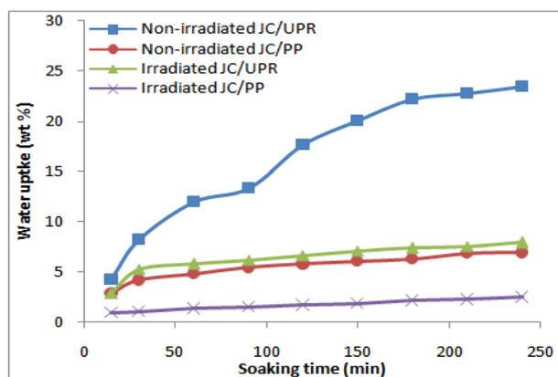
Figure 7. Water uptake of untreated and irradiated composites against soaking time
