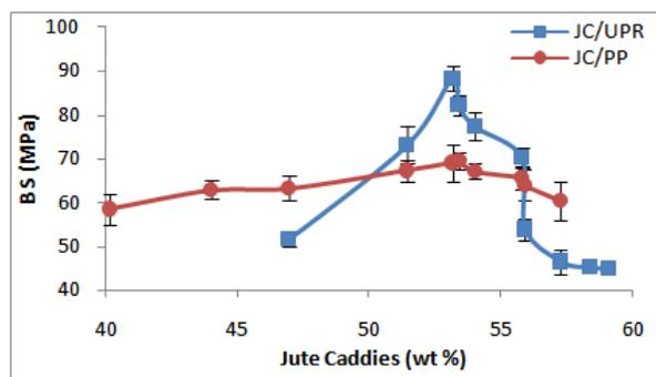
**Figure 3.** Bending strength of JC/UPR and JC/PP composites with fibre loading
