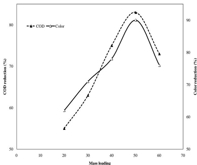
Figure 4. Effect of mass loading on COD and color at optimum pH=7
