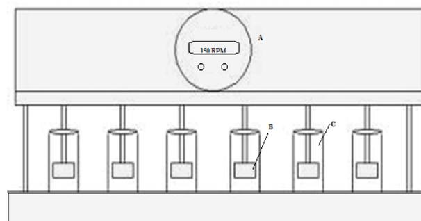
Figure 2. Jar test Apparatus
