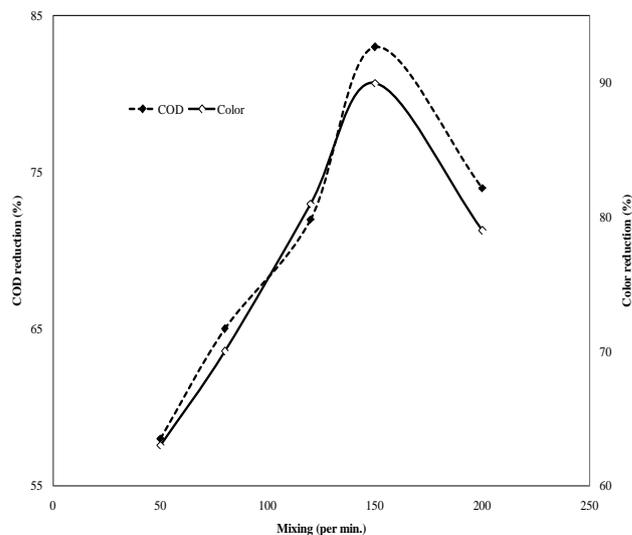
Figure 5. Effect of mixing on COD and color at optimum pH=7 and mass loading =50mm
