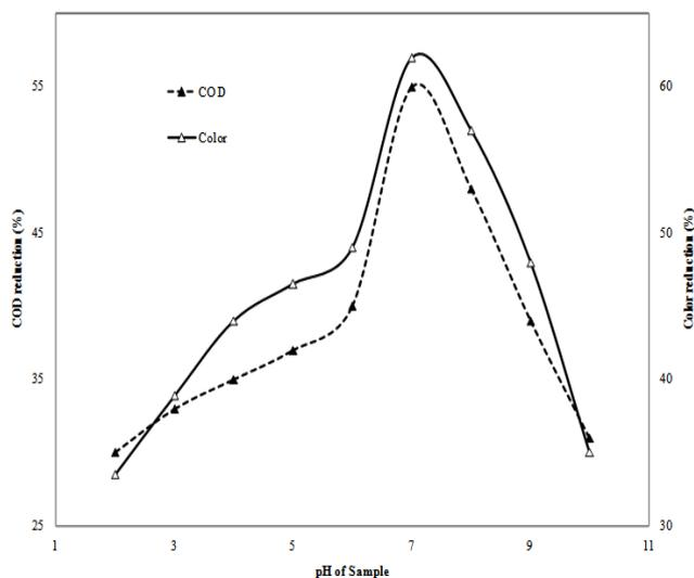
Figure 3. Effect of pH on COD and color reduction at pH<sub>i</sub> = 8.8, massloading = 20 mm
