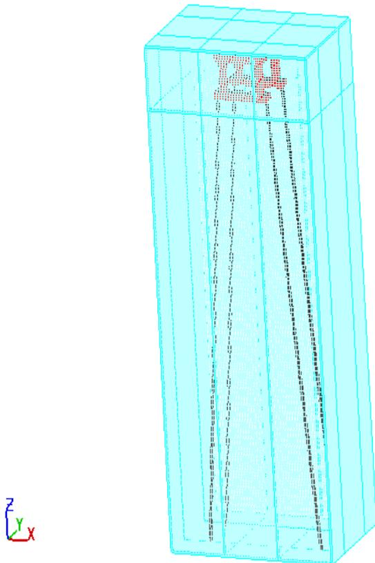
**Figure 2.** Meshing of semi submersible platform with 4 mooring lines
