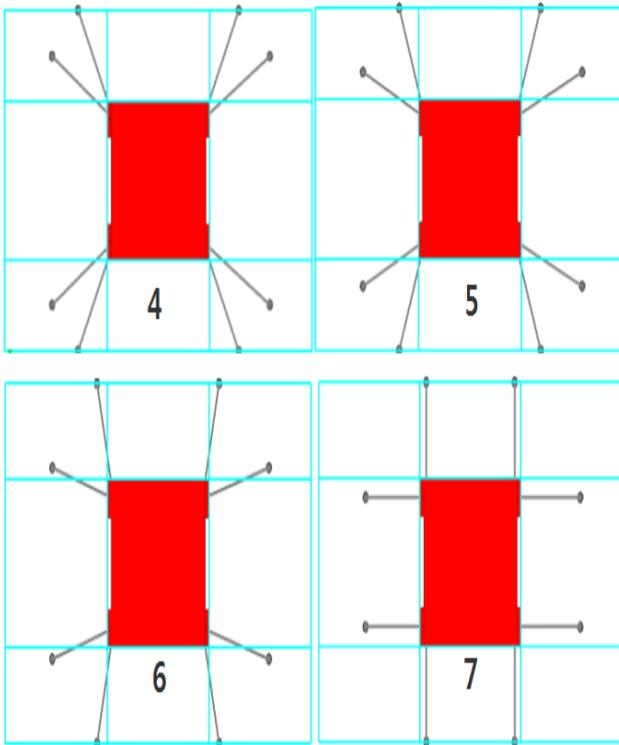
Figure 5. 4 kind of mooring system arrangement with 8 mooring lines
