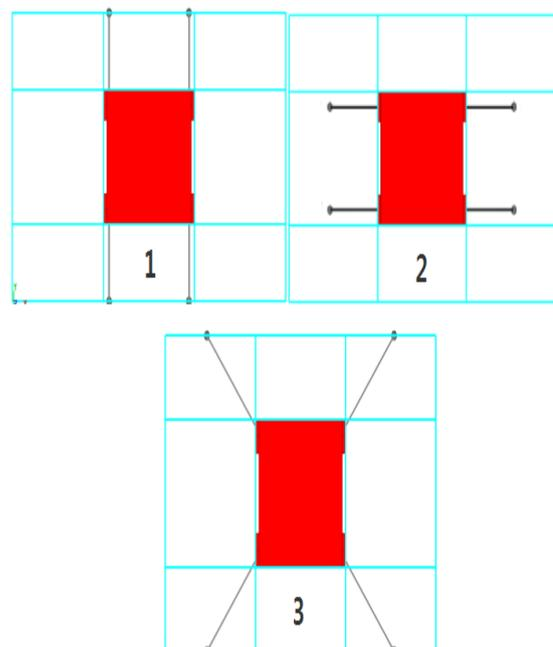
**Figure 4.** 3 kind of mooring system arrangement with 4 mooring lines
