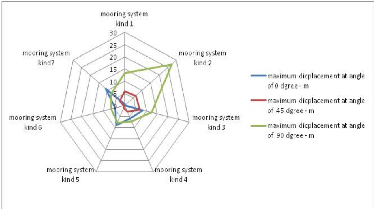
Figure 7. Semi-submersible platform Sway movement
