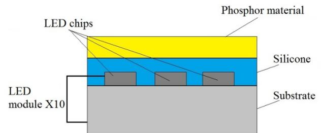
Figure 3. (Color online) Schematic view of the experimental LED module consisting of a blue LED chip and a PiG sample
