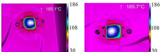
Figure 5. (Color online) Infrared images of the surface of the experimental LED modules with PiG samples #1 (left image) and #5 (right image). Temperature scale (in°C) is shown on the right of each image
