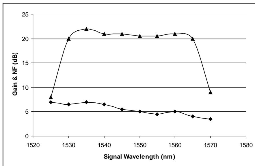
Figure 4. Gain and noise figure of hybrid Raman/Erbium-doped fiber amplifier (HFA) for different signal wavelengths
