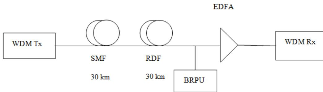
Figure 3. Schematic design of hybrid Raman/Erbium-doped fiber amplifier (HFA)
