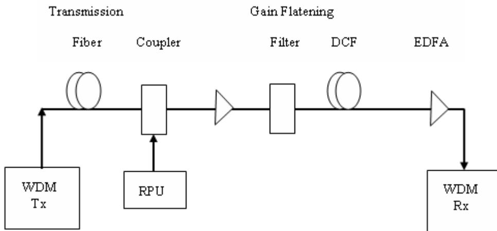
Figure 2. A typical hybrid Raman/Erbium-doped fiber amplifier. RPU stands for Raman pumping unit
