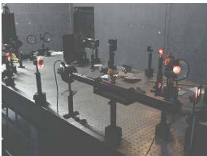
Figure 1. Holographic Lens recording setup
