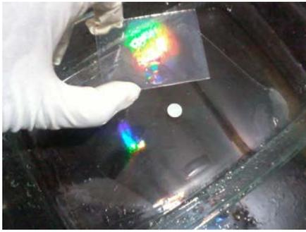
**Figure 3.** Recorded Holographic Lens
