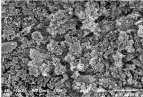
**Figure 2.** SEM micrograph of undoped ZnO
