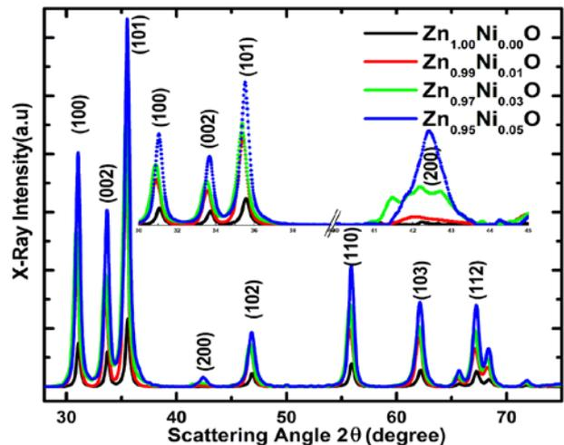
Figure 1. XRD spectra of Undoped and Ni-doped ZnO
