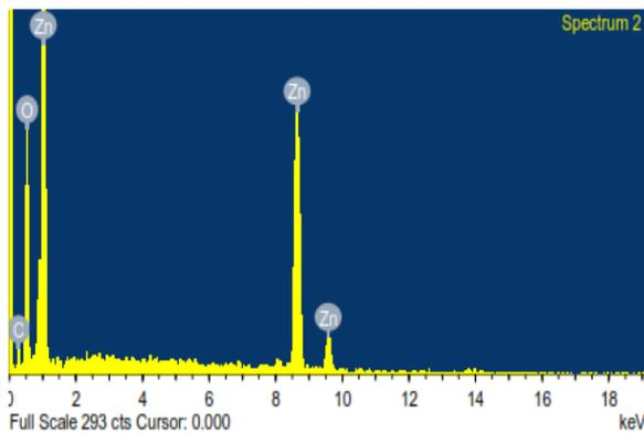
**Figure 3.** EDS spectra of undoped ZnO
