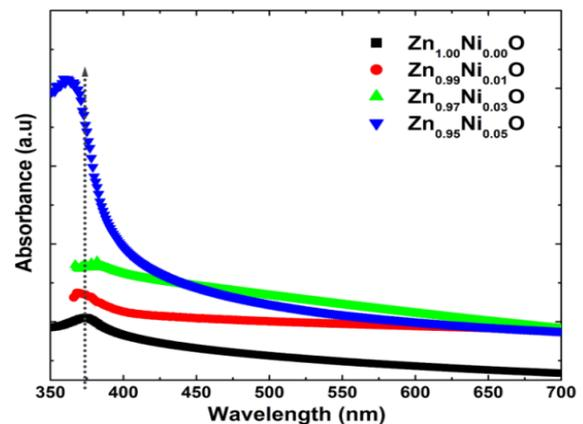
**Figure 5.** Absorbance spectra of undoped and Ni-doped ZnO
