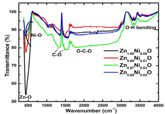
**Figure 4.** FTIR spectra on undoped and Ni-doped ZnO
