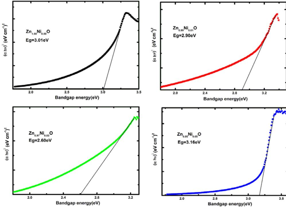
Figure 6. Band gap spectra of undoped and Ni ZnO NPs
