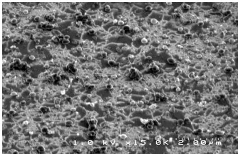
**Figure 4.** SEM image of CNTs fabricated on Si/SiO<sub>2</sub>/Co substrate
