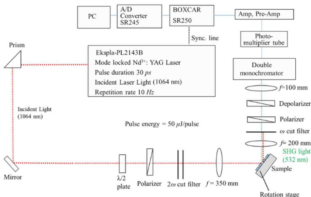
**Figure 1.** Optical setup for measuring SHG intensity from bare CNTs, CNTs/PEP with variant concentration of peptides and different wavelength tuned manually by using monochromator
