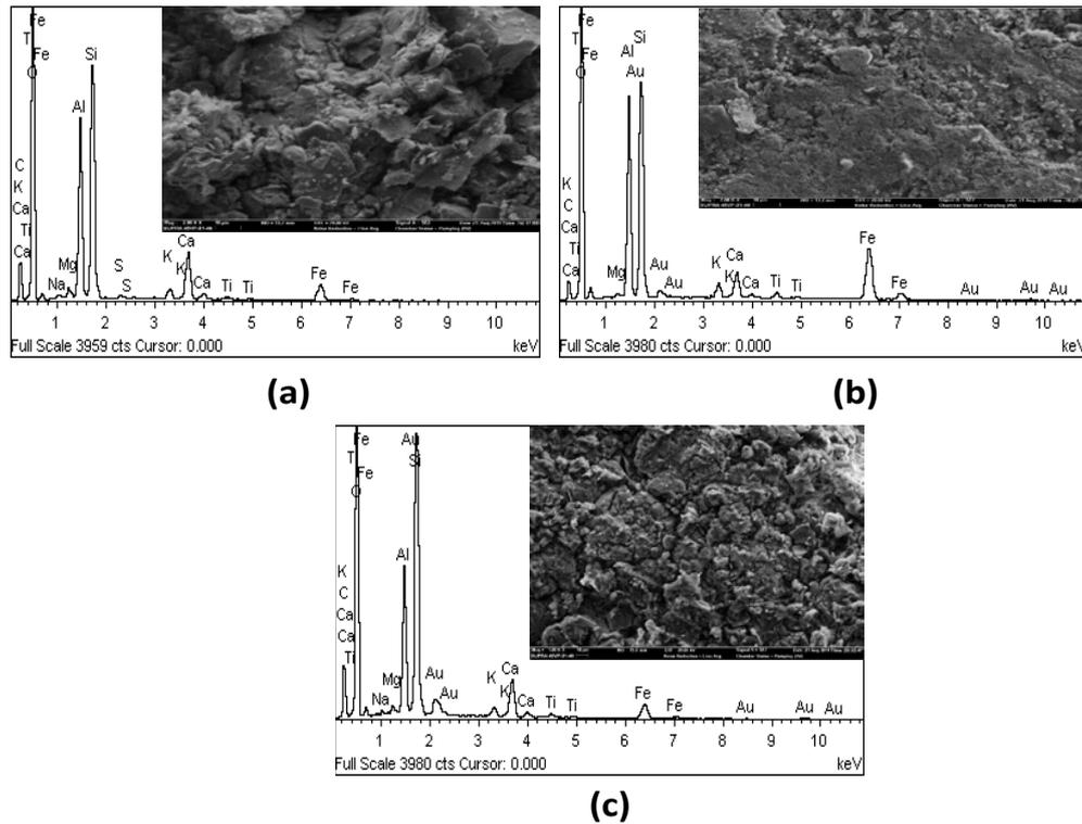
**Figure 6.** Microstructure and EDS analysis (a) formulation F91TK4C5; (b) formulation K89TK6C5; (c) formulation Y89TK6C5
