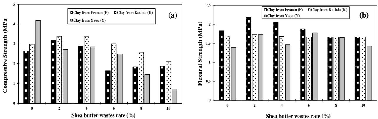
Figure 5. Mechanical resistance in compression (a) and in flexural (b) of CEB
