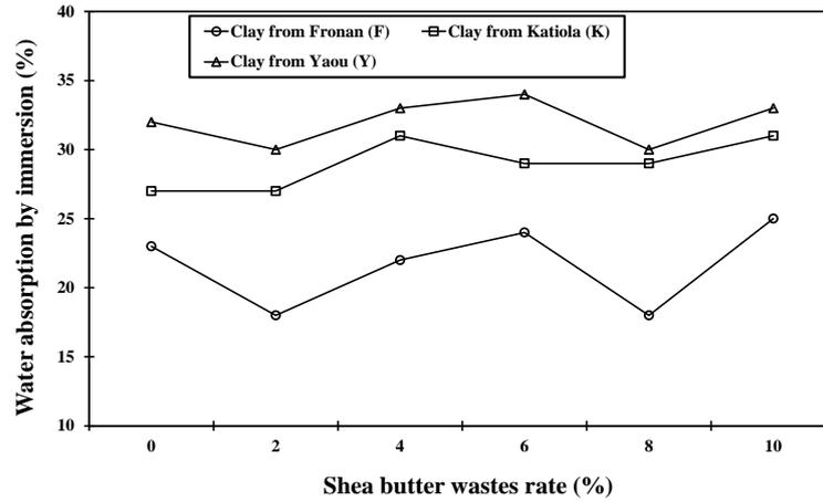
Figure 4. Total water absorption of CEB
