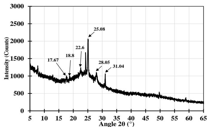
Figure 2. XRD pattern of shea waste
