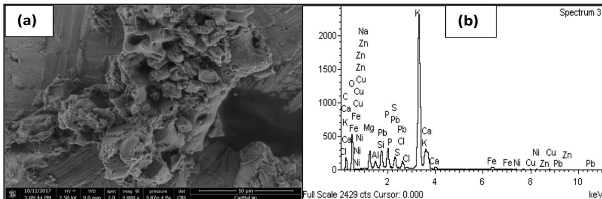
Figure 3. (a) SEM image; (b) energy dispersion spectrum of shea wastes
