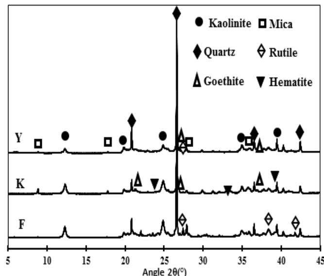
Figure 1. X-ray diffraction patterns of clay raw materials
