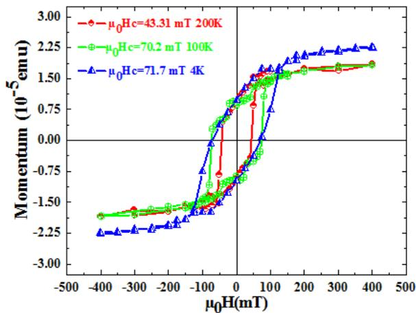
Figure 3. Hysteresis loops of Au/Co(0.7nm)/Au recorded at 200, 100 and 4 K, in polar configuration
