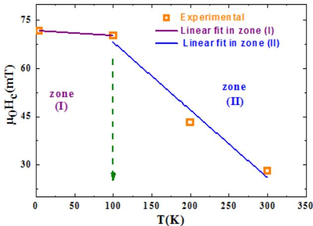
**Figure 5.** Fitting of coercive field depending on the temperature of Au/Co(0.7nm)/Au
