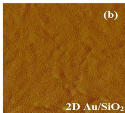
**Figure 1.** (a): XRD spectra of a 25 nm thick Au layers deposited on SiO<sub>2</sub> substrate. (b): 2D AFM image of a 25 nm thick Au buffer layer deposited on SiO<sub>2</sub> substrate
