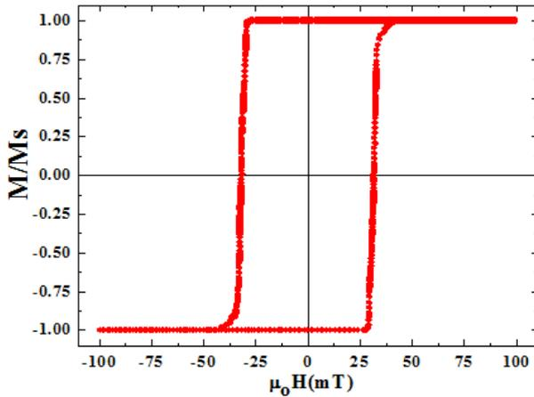
Figure 2. Quasistatic hysteresis loops of Au/Co(0.7 nm)/Au/SiO<sub>2</sub> measured at 300 K by PMOKE.
