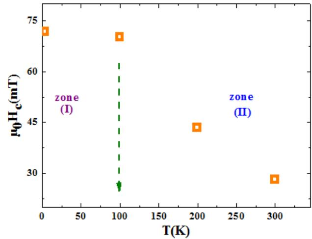
Figure 4. Coercive field depending on the temperature of Au/Co(0.7nm)/Au
