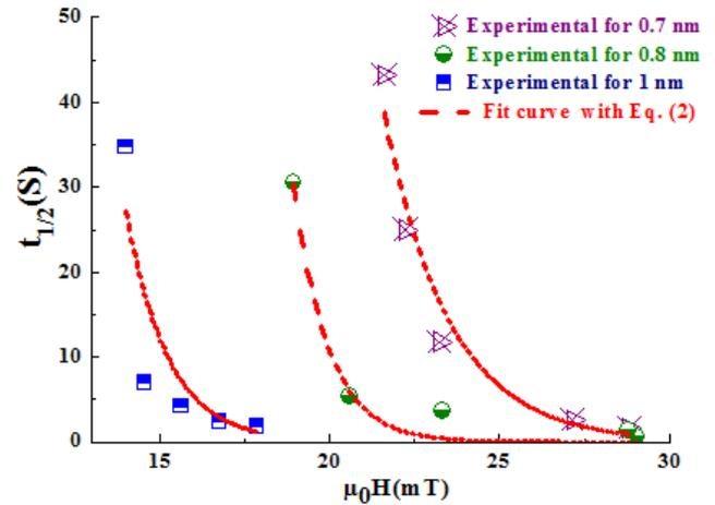
**Figure 2.**  $t_{1/2}$  depending on  $\mu_0 H$  and it fitting by Arrhenius-Néel law Eq. (2), for the three samples
