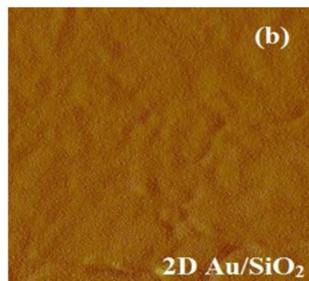
**Figure 1.** (a): XRD spectra of a 25 nm thick Au layers deposited on  $\text{SiO}_2$  substrate. (b): 2D AFM image of a 25 nm thick Au buffer layer deposited on  $\text{SiO}_2$  substrate
