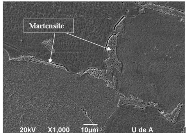
Figure 8. HAZ-F showing grain boundaries free of precipitates
