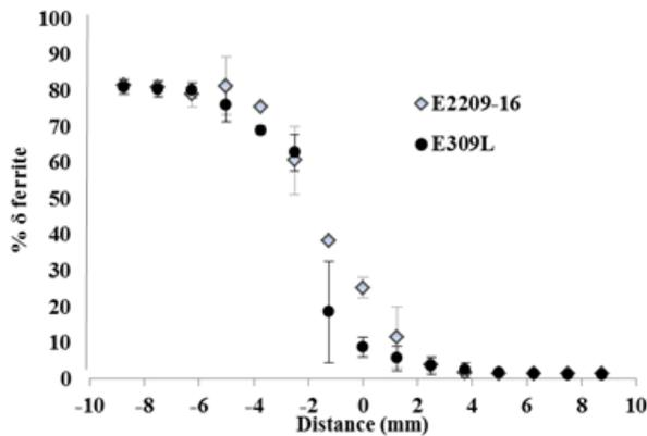
Figure 12. Delta ferrite profiles of the coupons
