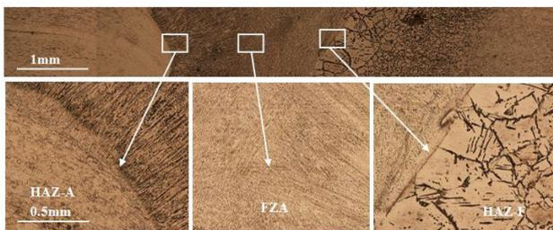
**Figure 1.** SMAW welding AISI 316L-AWS E309L-AISI 430
