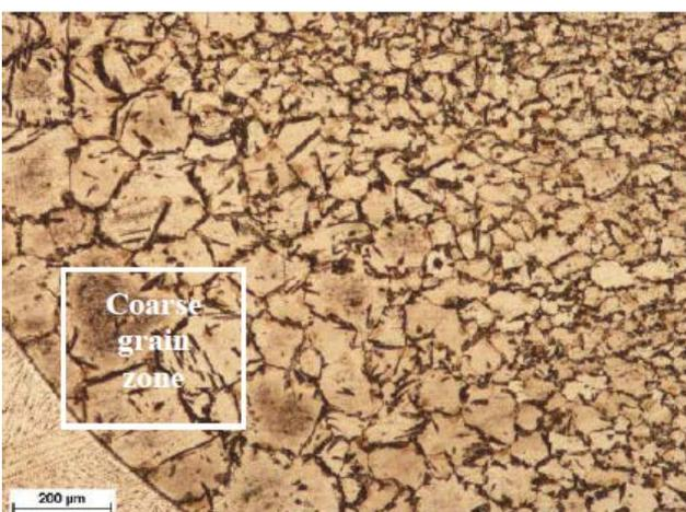
Figure 7. Microstructure of HAZ-F of AISI 430-AWS E309L
