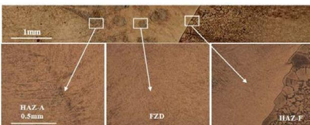
**Figure 2.** SMAW welding AISI 316L-AWS E2209-16-AISI 430
